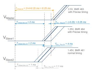
Figure A5. TON\_DELAY calculations for tracking master using Eq. A2.
