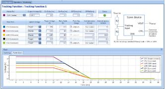
Efigure A19. Voltage tracking power-down configuration of 6 rails using Flex Power Designer design tool.
