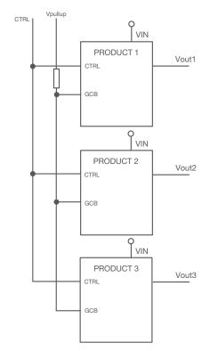
Figure 10 GCB Based Sequencing example – Enabling is shown generated via CTRL pin, but can also be done without a common CTRL by using PMBus OPERATION command.
