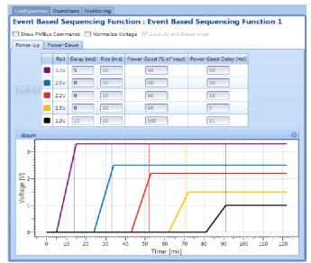
Figure A10. Event-based power-up sequencing configuration of 5 rails using Flex Power Designer design tool. The configured start-up time for all rails is 91 ms.
