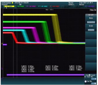
Figure A17. GCB-based down-sequencing accumulated variations from 100 power-down occasions of BMR 462-464. The CTRL signal, the bottom trace, triggers the start of all five rails. The configured total down-sequencing time is 90 ms. The achieved down-sequencing time, incl timing variation, is 105.0 – 118.0 ms. This is due to to the fact that the timing error in previous rails are accumulated. However, non-overlap is always granted in GCB-based sequencing. (20 ms/div).
