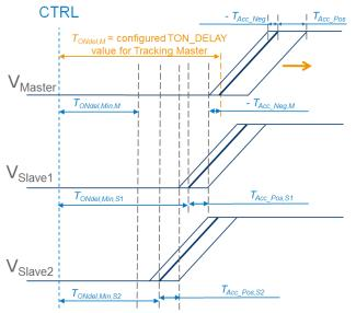
Figure A1. Calculation of smallest possible turn-on delay value of the master using Eq. A2.
