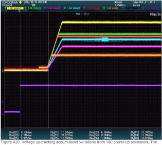
CTRL signal, the bottom trace, triggers the start of the tracking master rail. The tracking master, a BMR 463 0002/001 (3.3V) is configured with precise-ramp-up timing. As seen, the tracking slaves are following the master closely and the timing variation is small. The statistics are collected in Table A1. (20 ms/div).
