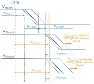
Figure A2. Calculation of smallest possible turn-off delay values of the slaves using Eq. A4.
