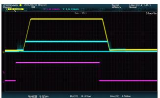
Figure 22 Coincident Tracking – Power-o/noff sequence of a BMR 464 as tracking master (TON\_DELAY = 10ms, TOFF\_DELAY = 0ms, Vout = 3.,3V in yellow color) and a BMR 465 as tracking slave (TON\_DELAY = 0 ms, TOFF\_DELAY = 35ms, Vout = 1V in light blue color) CTRL signal is shown in lilac color. The oscillscope plot shows 100 accumulated tests. (*x*-scale is 20 ms/div).
