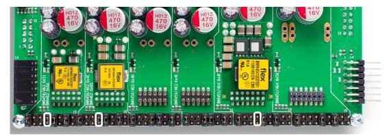
Figure 15. Setting up 3E POL Board (ROA 128 3836) jumpers for GCB Based Sequencing.
