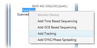
Figure 17 Adding Voltage Tracking Function.
