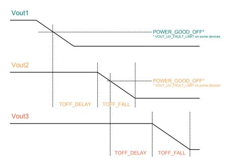
Fig 9b Event based down-sequencing – Illustration of which settings to be made in which rail. The total time between the Preceding rail, Vout1, and the following rail, Vout2, is determined as follows: Vout1 are configured using POWER\_GOOD\_OFF (or VOUT\_UV\_FAULT\_LIMIT) while Vout2 is configured using TOFF\_DELAY and TOFF\_FALL.
