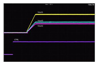
Figure 21 Tracking - Turn-on sequence example.( x-scale is 10 ms/div)
