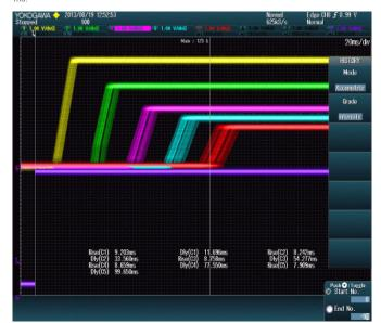
Figure A16. GCB-based up-sequencing accumulated variations from 100 power-up occasions, of BMR 462-464. The CTRL signal, the bottom trace, triggers the start of all five rails. The configured total up-sequencing time is 98 ms. The achieved timing variation of the last rail is quite large in this example, 94.5 – 106.5 ms. This is due to the fact that the timing error in previous rails are accumulated. However, non-overlap is always granted in GCB-based sequencing. (20 ms/div).
