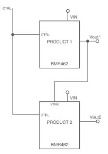
Figure 16 Voltage Tracking Configuration.
