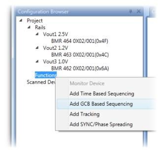
Figure 12. Adding GCB Based Sequencing
