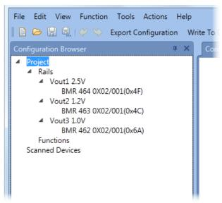
Figure 11. Rails for Example 3 in Flex Power Designer. Without any sequencing added yet, this is the same Rail setup as in Example 1
