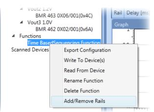
Figure 5. Adding Rails to the Sequencing Function.
