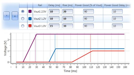
Figure 14a. GCB Based Power-Up Sequencing. There arrow buttons allow one to change the sequencing order.
