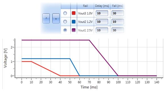
Figure 14b. GCB Based Power-Up Sequencing. There arrow buttons allow one to change the sequencing order.
