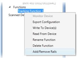
Figure 18. Adding rails to tracking function.
