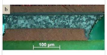
Picture 4: Cross polarized image of a 30 mil SAC305 LGA solder joint exhibiting an interlaed twinned grain structure
