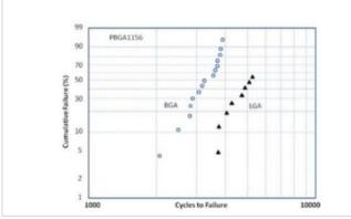
Picture 2: Weibull plot showing cycles to failure in -40°/125°C thermal cycling – SAC305 PBGA1156 and LGA 1156
