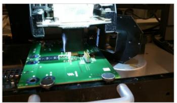
Picture 10: Reflow station with air nozzle
