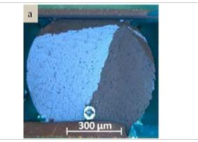
Picture 3: Cross polarized image of a 30 mil SAC305 BGA solder joint demonstrating the characteristic 'Beach Ball' microstructure.
