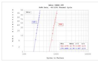
Picture 1: Weibull plot showing cycles to failure in -40°/125°C thermal cycling – Sn/Pb BGAs and corresponding LGAs
