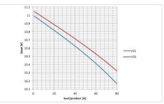
Figure 10: Predicted worst case current share with 4.5  $\sigma$  output voltage difference at 0 A and +3  $\sigma$  on RO1 and -3  $\sigma$  on RO2. R<sub>th</sub>=1.4 K/W. Ambient temperature is 40°C for both products. V<sub>in</sub>  $\geq$  51 V.
