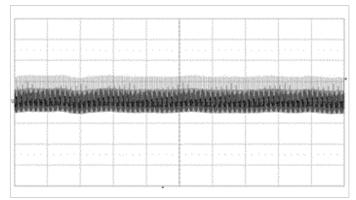
Figure 6b: Output ripple single product 100 µs/div, 20 mV/div
