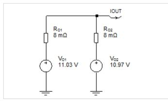
Figure 2: A simplified schematic model of two parallel PKM4817LNH
