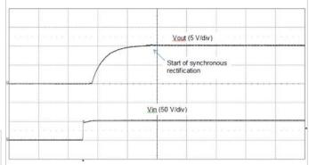
Figure 4: Start-up for two parallel products with 152 A resistive load and  $C_{out}$  = 10 mF. (5 ms/div)
