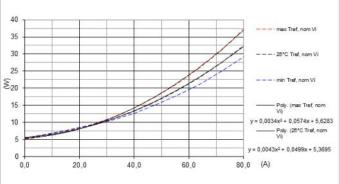
Figure 3: measured power dissipation,  $P_d$  vs output current for  $T_{P1}$ = -30, 25 and 90°C.
