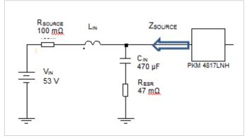
Figure 5: Source impedance and external input capacitance
