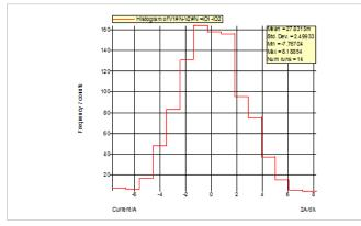
Figure 6a: Monte Carlo 1 k runs. Histogram of statistical output current difference (on x-axis) at a total output current of 160 A.  $T_{P1}$  is around 90°
