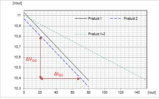
Figure 1: Typical output current from two products with 60mV output voltage initial setting tolerances but with equal output resistance.
