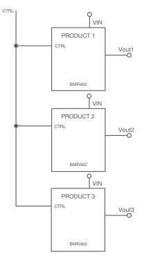
The configuration procedure for time based sequencing is straightforward. It only includes configurations of four registers, TON\_DELAY, TON\_RISE, TOFF\_DELAY, and TOFF\_FALL for all products/rails in the sequencing group.
