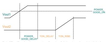
Fig 3a GCB and Event based up-sequencing – Illustration of which settings to be made in which rail. The total time between the Preceding rail, Vout1, and the following rail, Vout2, is determined as follows: Vout1 are configured using POWER\_GOOD\_ON and POWER\_GOOD\_DELAY while Vout2 are configured using TON\_DELAY and TON\_RISE.
