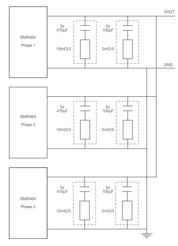
Figure 18. 3-phase current sharing example.
