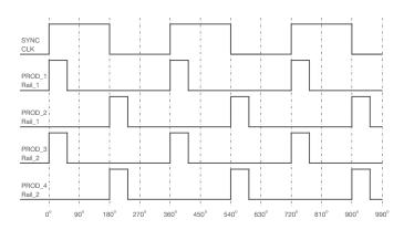
Figure 11. Timing diagram for a 2 rail x 2-phase current sharing example.
