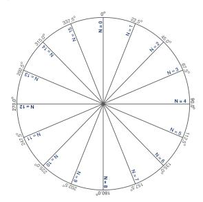
Figure 5. Phase offset resolution wheel.
