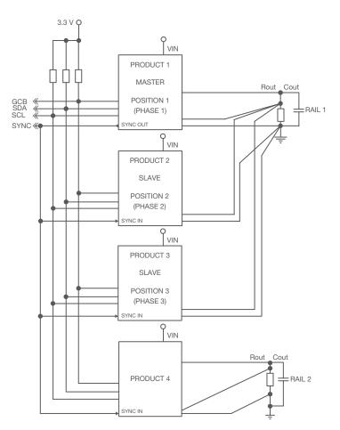
Figure 8. Example of sharing group and auxiliary output rail with a common SYNC clock.
