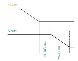
Fig 5 GCB based down-sequencing – Illustration of which settings to be made in which rail. The total time between the Preceding rail, Vout1, and the following rail, Vout2, is determined as follows: When Vout2 has reached 0 V, the start of Vout1 triggers. Vout1 are configured using TOFF\_DELAY and TOFF\_FALL.
