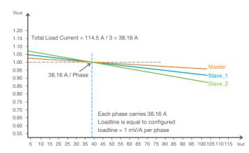
Figure 2. Balanced phase currents. Slave reference voltage(s) is trimmed until all products' currents equalize.
