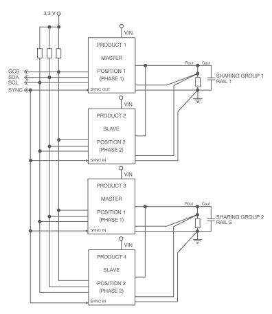
Figure 10. Example of 2 x 2-phase current sharing groups using the same SYNC clock.
