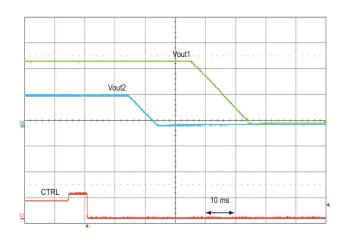
Figure 6b GCB-based sequencing example – Turn-off.
