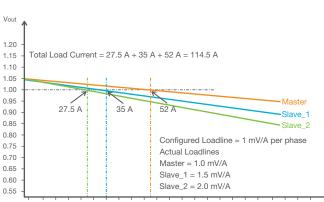
5 10 15 20 25 30 35 40 45 50 55 60 65 70 75 80 85 90 95 100105110115 lout Figure 1. Unbalanced phase currents due to slope error.
