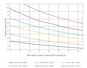
Figure 21. Recommended maximum individual droop per phase vs VOUT and max IOUT for BMR463.
