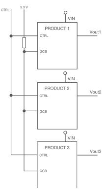
Figure 4 GCB Based Sequencing example – Enabling is generated via CTRL pin
