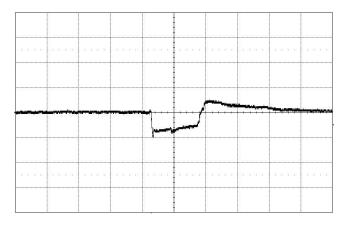
Figure 7. Example of output voltage deviation during drop (10 mV/div, 10 ms/div)
