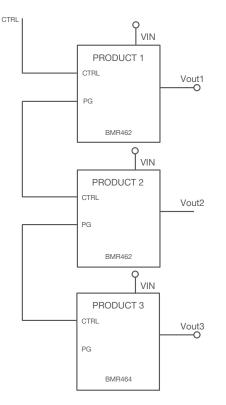
Figure 2 Event based sequencing example. A change of sequencing order will require a hardware re-configuration. Using the Event based method, i.e. connecting PG to CTRL, as shown in Figure 2, the same order for start-up and shut-down are provided. This method requires a hardware modification if the sequence order is changed.
