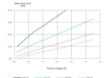
Figure 22. Max ramp time vs output voltage and switch frequency
