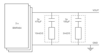
Figure 19. Current sharing compensation model..
