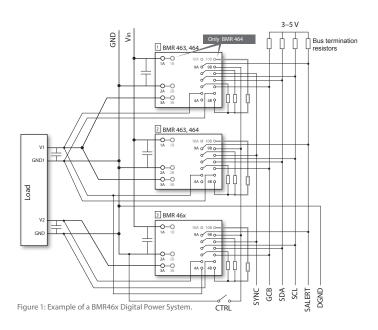
In this example of a typical system that uses the BMR46x series, regulators no 1 and no 2 are in current sharing mode (only BMR463 and BMR464) supplying rail V1 with up to 80 A. Regulator no 3 is in voltage tracking mode, making rail V2 track rail V1. All three regulators are synchronized via the SYNC signal, which can be generated internally or taken from an external source. Using phase spreading will reduce the current ripple on input rail Vin.
