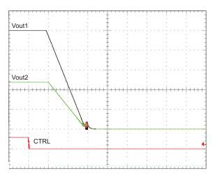
Figure 10 Tracking - Turn-on sequence example.( x-scale is 10 ms/div)
