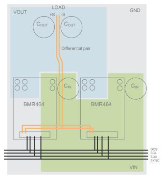
Figure 17. Layout example, two products.
