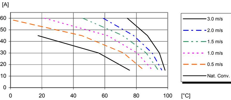
Available load current vs. ambient air temperature and airflow at  $V_i = 48$  V. See Thermal Consideration section.
