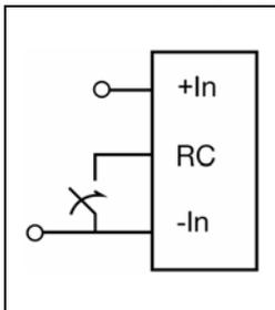
The product is fitted with a remote control function referenced to the primary negative input connection (-In). The RC function allows the product to be turned on/off by an external device like a semiconductor or mechanical switch. The RC pin has an internal pull up resistor to internal voltage reference 18V.
