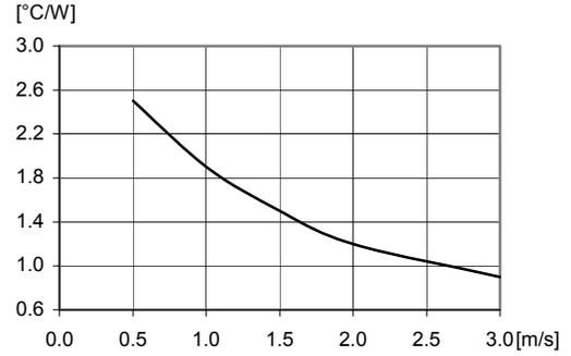
Thermal resistance vs. airspeed measured at the converter. Tested in wind tunnel with airflow and test conditions as per the Thermal consideration section.  $V_i = 48$  V,  $I_{out} = 60$  A.
