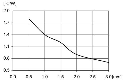
Thermal resistance vs. airspeed measured at the converter. Tested in wind tunnel with airflow and test conditions as per the Thermal consideration section.  $V_i = 48$  V,  $I_{out} = 60$  A. The type of heat sink is AAVID 241402B92200G
