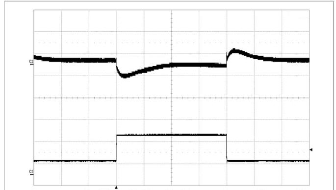
Output voltage response to load current step-
