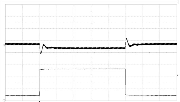
Output voltage response to load current step-change (22.5-67.5-22.5 A) at:
