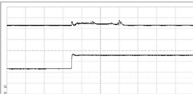
Output voltage response to input voltage transient at:  $T_{P1} = +25^\circ\text{C}$ ,  $V_1 = 36-60\text{ V}$ ,
