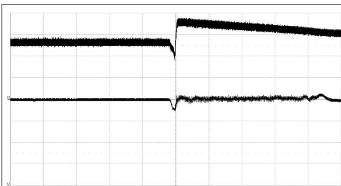
Output voltage response to input voltage
