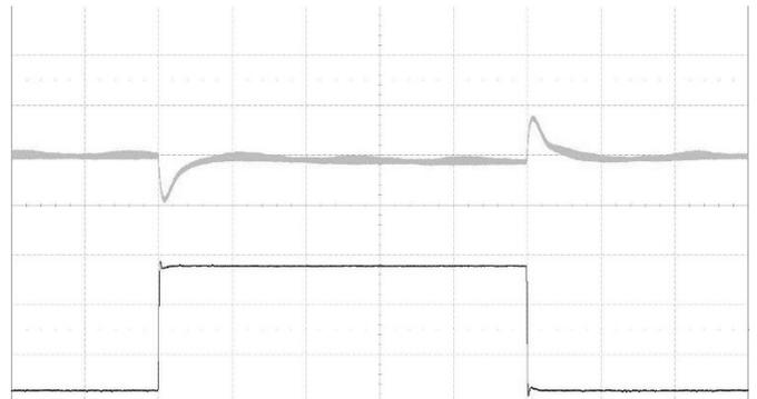
Output voltage response to load current step-
