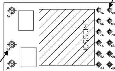
Pin 2A for measurement of minimum Pin (solder joint) temperature  $T_{PIN}$
