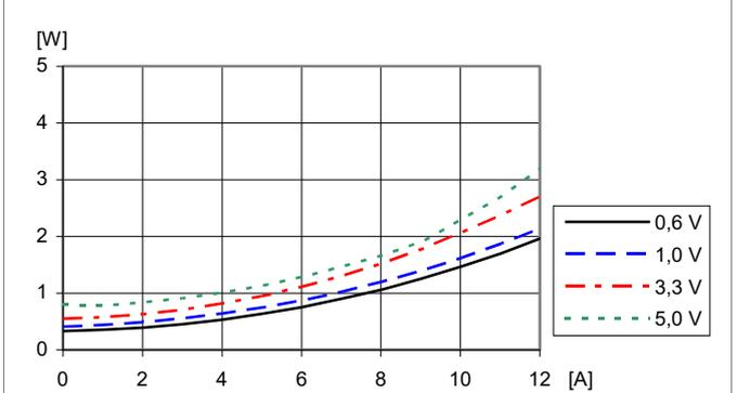
Dissipated power vs. load current and output voltage:
