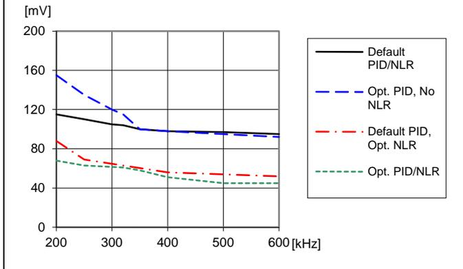
Load transient peak voltage deviation vs. frequency. Step-change (3-9-3 A).  $T_{P1} = +25^{\circ}\text{C}$ ,  $V_I = 12\text{ V}$ ,  $V_O = 3.3\text{ V}$ ,  $C_O = 470\text{ }\mu\text{F}/10\text{ m}\Omega$
