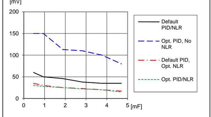
Load transient peak voltage deviation vs. decoupling capacitance. Step-change (3-9-3 A). Parallel coupling of capacitors with  $470\text{ }\mu\text{F}/10\text{ m}\Omega$ ,  $T_{P1} = +25^{\circ}\text{C}$ ,  $V_I = 12\text{ V}$ ,  $V_O = 1.0\text{ V}$ ,  $f_{sw} = 320\text{ kHz}$ ,  $di/dt = 2\text{ A}/\mu\text{s}$
