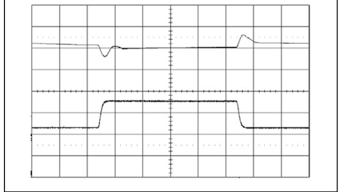
Output voltage response to load current step-change (3-9-3 A) at:  $T_{P1} = +25^{\circ}\text{C}$ ,  $V_I = 12\text{ V}$ ,  $V_O = 3.3\text{ V}$ ,  $di/dt = 2\text{ A}/\mu\text{s}$ ,  $f_{sw} = 320\text{ kHz}$ ,  $C_O = 470\text{ }\mu\text{F}/10\text{ m}\Omega$ . Default PID Control Loop and NLR. Top trace: output voltage (200 mV/div.). Bottom trace: load current (5 A/div.). Time scale: (0.1 ms/div.).
