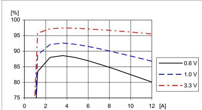
Efficiency vs. load current and output voltage:
