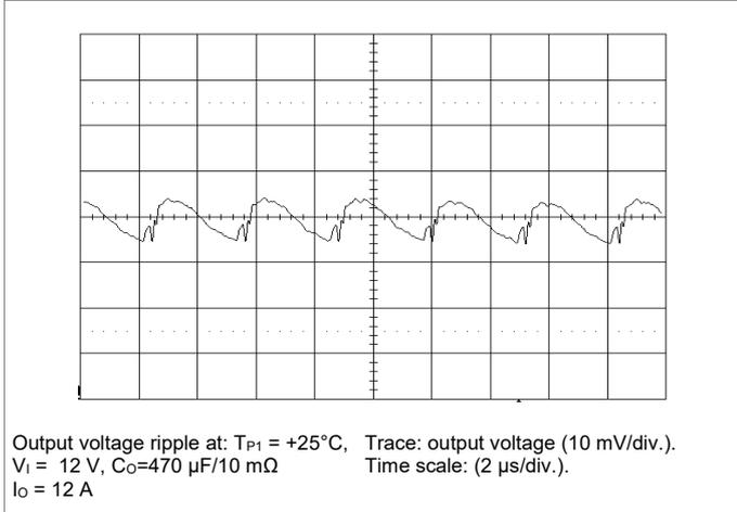
**Output Ripple & Noise,  $V_o=3.3\text{ V}$**
