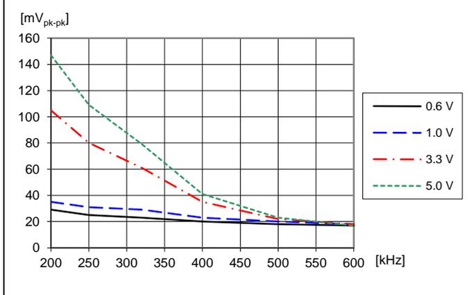
Output voltage ripple  $V_{pk-pk}$  at:  $T_{P1} = +25^{\circ}\text{C}$ ,  $V_I = 12\text{ V}$ ,  $C_O = 470\text{ }\mu\text{F}/10\text{ m}\Omega$ ,  $I_O = 12\text{ A}$  resistive load. Default configuration except changed frequency.
