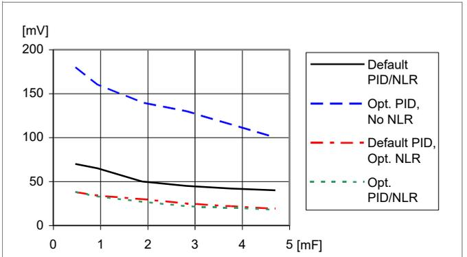
Load transient peak voltage deviation vs. external capacitance. Step-change (3-9-3 A). Parallel coupling of capacitors with 470  $\mu$ F/10 m $\Omega$ ,  $T_{P1} = +25^\circ$ C.  $V_i=12$  V,  $V_O=3.3$  V,  $f_{sw}=320$  kHz,  $di/dt=2$  A/ $\mu$ s
