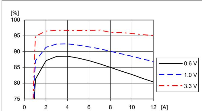
Efficiency vs. load current and output voltage:
