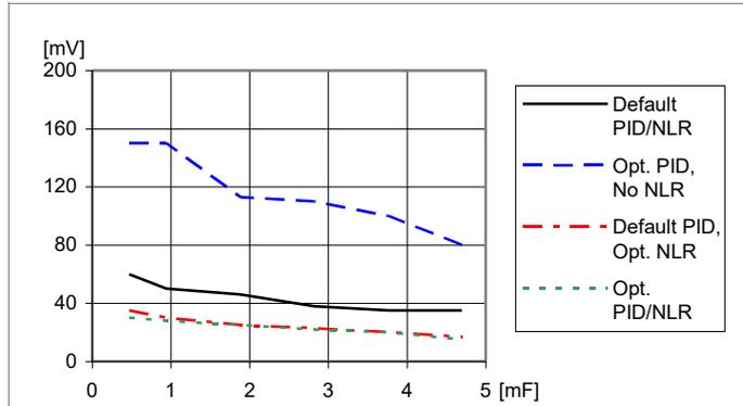
Load transient peak voltage deviation vs. external capacitance. Step-change (3-9-3 A). Parallel coupling of capacitors with 470  $\mu$ F/10 m $\Omega$ ,  $T_{P1} = +25^\circ$ C.  $V_i=12$  V,  $V_O=1.0$  V,  $f_{sw}=320$  kHz,  $di/dt=2$  A/ $\mu$ s
