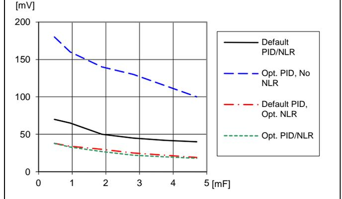
Load transient peak voltage deviation vs. decoupling capacitance. Step-change (3-9-3 A). Parallel coupling of capacitors with  $470\text{ }\mu\text{F}/10\text{ m}\Omega$ ,  $T_{P1} = +25^{\circ}\text{C}$ ,  $V_I = 12\text{ V}$ ,  $V_O = 3.3\text{ V}$ ,  $f_{sw} = 320\text{ kHz}$ ,  $di/dt = 2\text{ A}/\mu\text{s}$
