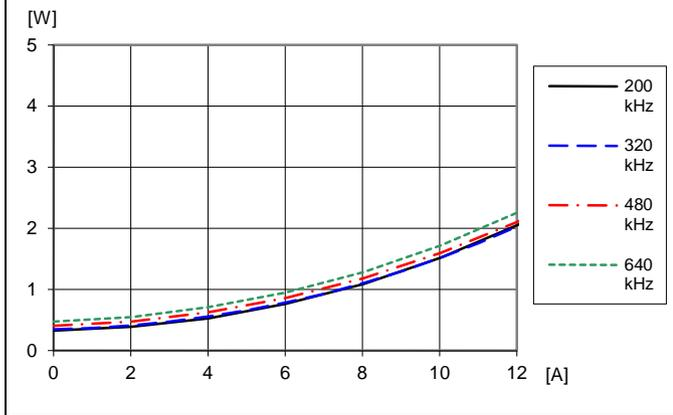
Dissipated power vs. load current and switching frequency at  $T_{P1} = +25^{\circ}\text{C}$ ,  $V_I = 12\text{ V}$ ,  $V_O = 3.3\text{ V}$ ,  $C_O = 470\text{ }\mu\text{F}/10\text{ m}\Omega$ . Default configuration except changed frequency
