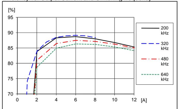
Efficiency vs. load current and switching frequency at T<sub>P1</sub> = +25°C. V<sub>I</sub>=12 V, V<sub>O</sub>=3.3V, C<sub>O</sub>=470 μF/10 mΩ
