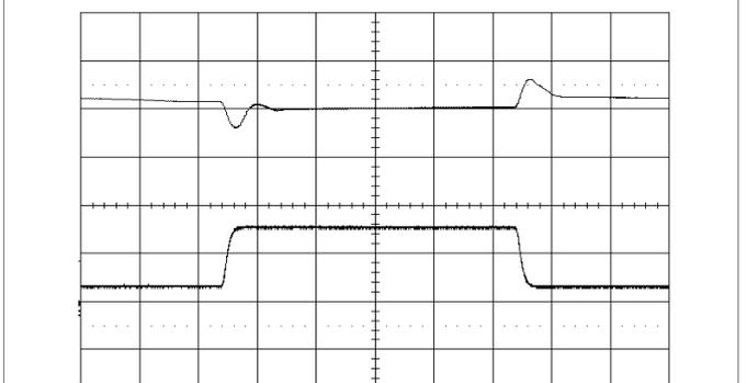
Output voltage response to load current step-change (3-9-3 A) at:  $T_{P1} = +25^\circ$ C,  $V_i = 12$  V,  $V_O = 3.3$  V,  $di/dt=2$  A/ $\mu$ s,  $f_{sw}=320$  kHz,  $C_O=470$   $\mu$ F/10 m $\Omega$
