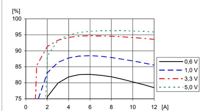
Efficiency vs. load current and output voltage at
