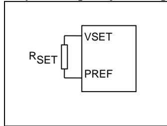
Using an external Pin-strap resistor,  $R_{SET}$ , the output voltage can be set in the range 0.6 V to 3.3 V at 28 different levels shown in the table below. The resistor should be applied between the VSET pin and the PREF pin.
