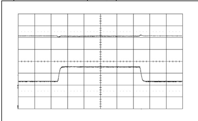
Output voltage response to load current step-change (3-9-3 A) at:
