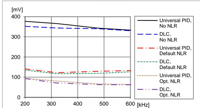
Load transient peak voltage deviation vs. frequency.
