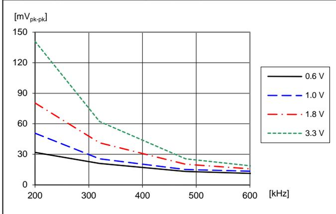
Output voltage ripple  $V_{pk-pk}$  at:  $T_{P1} = +25^\circ\text{C}$ ,  $V_I = 12\text{ V}$ ,  $C_O = 470\ \mu\text{F}/10\text{ m}\Omega$ ,  $I_O = 25\text{ A}$  resistive load. Default configuration except changed frequency.
