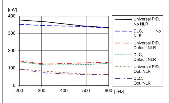
Load transient peak voltage deviation vs. frequency. Step-change (6.25-18.75-6.25 A).  $T_{P1} = +25^\circ\text{C}$ ,  $V_I = 12\text{ V}$ ,  $V_O = 1.0\text{ V}$ ,  $C_O = 470\ \mu\text{F}/10\text{ m}\Omega$
