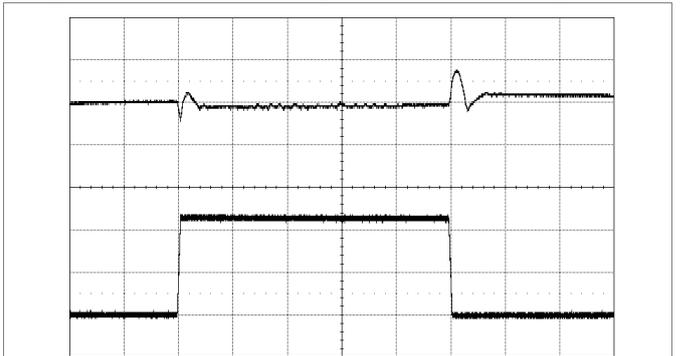
Output voltage response to load current
