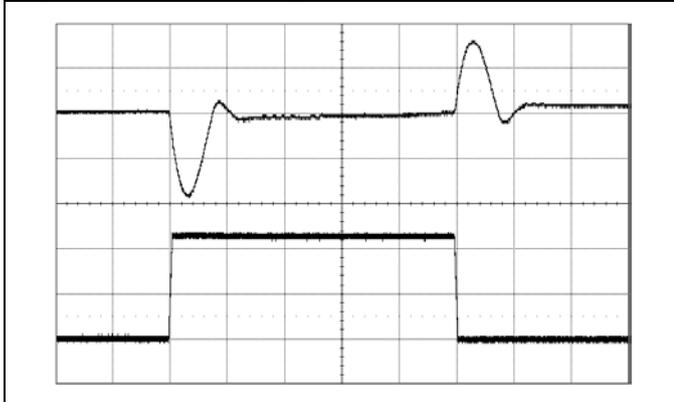
Output voltage response to load current step-change (6.25-18.75-6.25 A) at:
