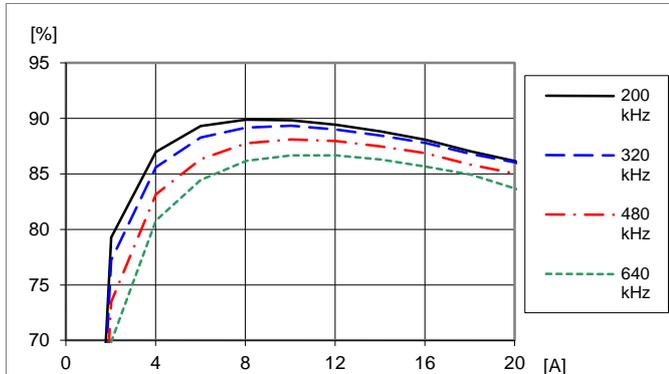
Efficiency vs. load current and switch frequency at
