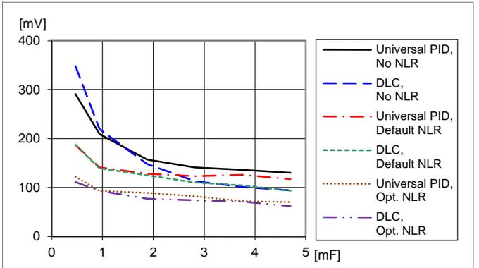
Load transient peak voltage deviation vs. external capacitance.
