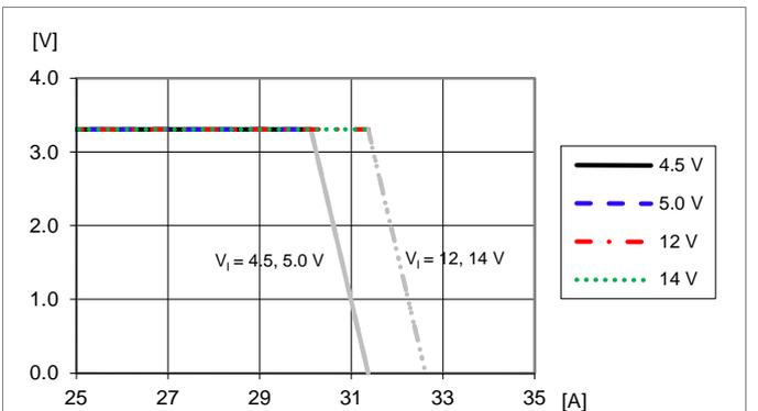
Output voltage vs. load current at  $T_{P1} = +25 ^\circ C$ ,  $V_o = 1.0 V$ .
