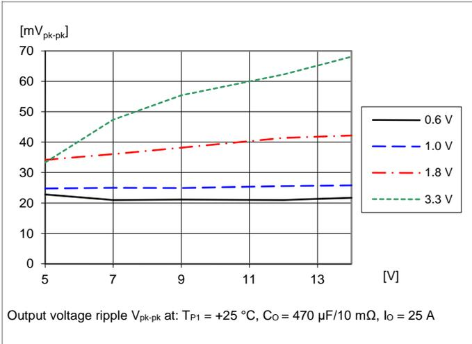
**Output Ripple vs. Frequency**
