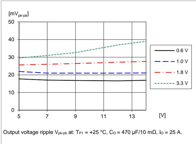
**Output Ripple vs. Frequency**
