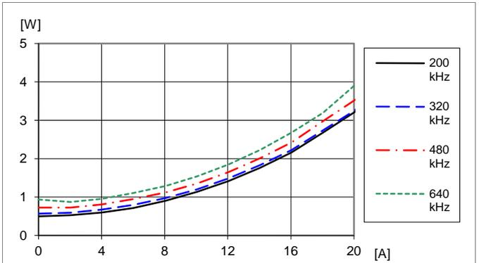
Dissipated power vs. load current and switch frequency at
