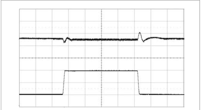
Output voltage response to load current step-change (5-15-5 A) at:  $T_{P1} = +25\text{ }^\circ\text{C}$ ,  $V_I = 12\text{ V}$ ,  $V_O = 1.0\text{ V}$ ,  $di/dt = 2\text{ A}/\mu\text{s}$ ,  $f_{sw} = 320\text{ kHz}$ ,  $C_O = 470\text{ }\mu\text{F}/10\text{ m}\Omega$
