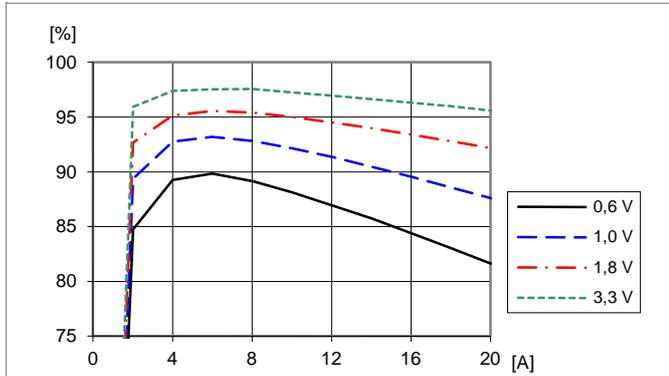
Efficiency vs. load current and output voltage:
