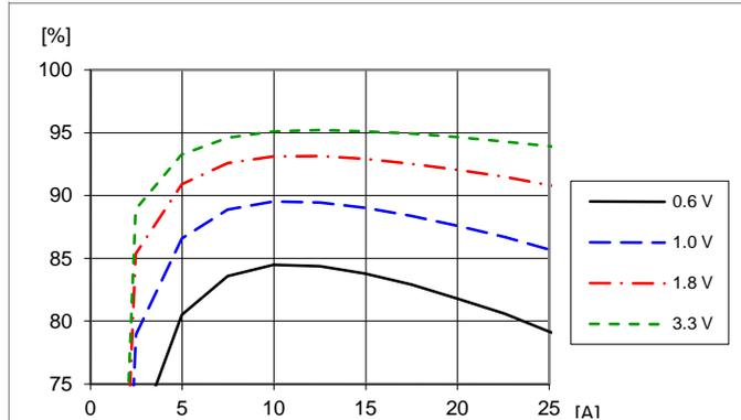
Efficiency vs. load current and output voltage at
