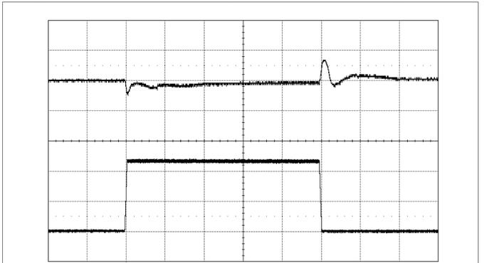
Output voltage response to load Step-change (6.25-18.75-6.25 A) at:  $T_{P1} = +25^\circ C$ ,  $V_I = 12 V$ ,  $V_O = 1.0 V$ ,  $di/dt = 2 A/\mu s$ ,  $f_{sw} = 320 kHz$ ,  $C_O = 470 \mu F/10 m\Omega$
