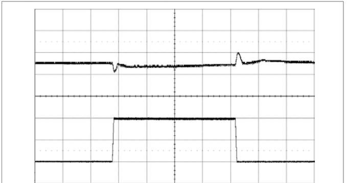
Output voltage response to load current step-change (5-15-5 A) at:  $T_{P1} = +25$   $^{\circ}$ C,  $V_I = 12$  V,  $V_O = 1.0$  V,  $di/dt = 2$  A/ $\mu$ s,  $f_{sw} = 320$  kHz,  $C_O = 470$   $\mu$ F/10 m $\Omega$
