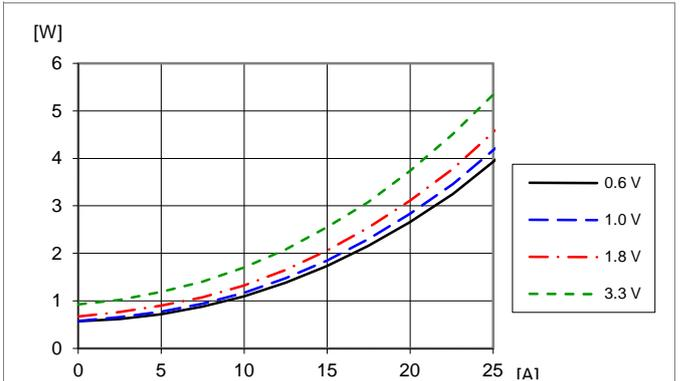
Dissipated power vs. load current and output voltage:
