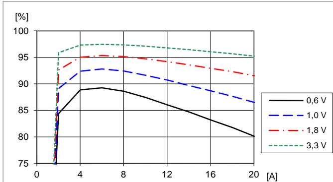
Efficiency vs. load current and output voltage:
