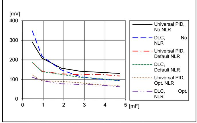
Load transient peak voltage deviation vs. decoupling capacitance. Step (6.25-18.75-6.25 A). Parallel coupling of capacitors with  $470\ \mu\text{F}/10\text{ m}\Omega$ ,  $T_{P1} = +25^\circ\text{C}$ ,  $V_I = 12\text{ V}$ ,  $V_O = 3.3\text{ V}$ ,  $f_{sw} = 320\text{ kHz}$ ,  $di/dt = 2\text{ A}/\mu\text{s}$
