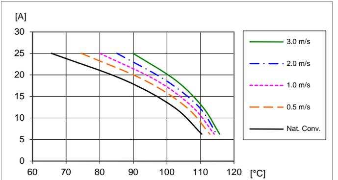
Available load current vs. ambient air temperature and airflow at  $V_o = 0.6 V$ ,  $V_i = 12 V$ . See Thermal Consideration section.
