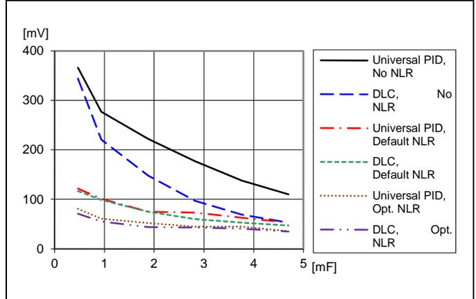
Load transient peak voltage deviation vs. decoupling capacitance. Step (6.25-18.75-6.25 A). Parallel coupling of capacitors with  $470\ \mu\text{F}/10\text{ m}\Omega$ ,  $T_{P1} = +25^\circ\text{C}$ ,  $V_I = 12\text{ V}$ ,  $V_O = 1.0\text{ V}$ ,  $f_{sw} = 320\text{ kHz}$ ,  $di/dt = 2\text{ A}/\mu\text{s}$
