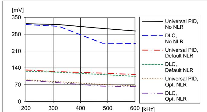
Load transient peak voltage deviation vs. frequency.
