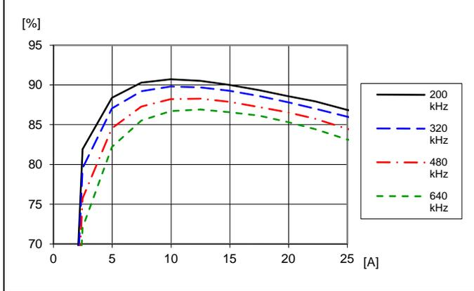
Efficiency vs. load current and switching frequency at  $T_{P1} = +25^\circ\text{C}$ ,  $V_I = 12\text{ V}$ ,  $V_O = 1.0\text{ V}$ ,  $C_O = 470\ \mu\text{F}/10\text{ m}\Omega$ . Default configuration except changed frequency
