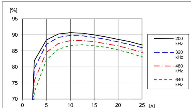
Efficiency vs. load current and switch frequency at
