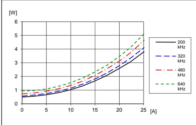
Dissipated power vs. load current and switching frequency at  $T_{P1} = +25^\circ\text{C}$ ,  $V_I = 12\text{ V}$ ,  $V_O = 1.0\text{ V}$ ,  $C_O = 470\ \mu\text{F}/10\text{ m}\Omega$ . Default configuration except changed frequency
