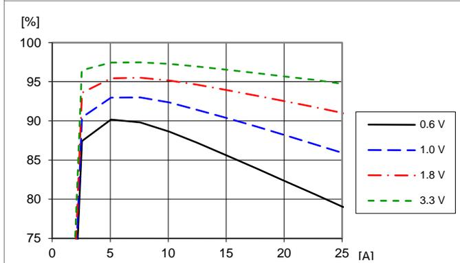
Efficiency vs. load current and output voltage:
