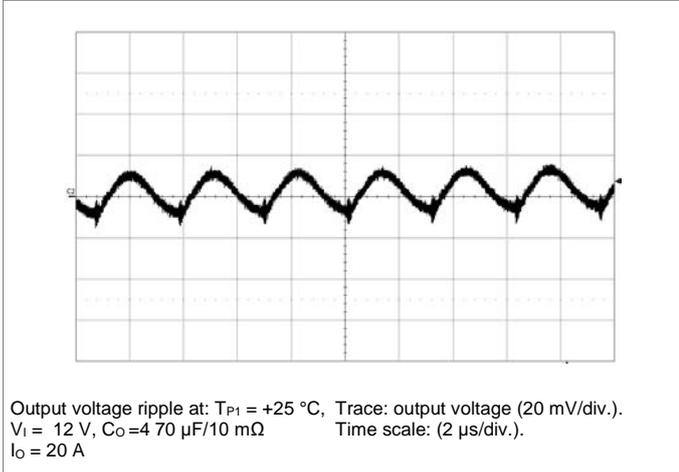
**Output Ripple & Noise,  $V_o = 3.3\text{ V}$**
