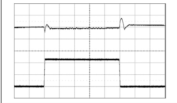
Output voltage response to load current step-change (6.25-18.75-6.25 A) at:
