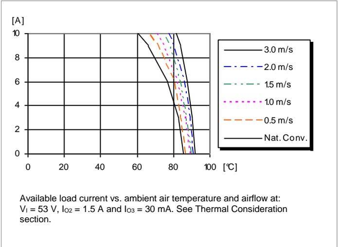
**Output Current Derating, Basic Insulation (P\*)**
