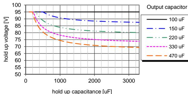
The chart shows maximum allowed hold up voltage and hold up capacitor at different output capacitors.
