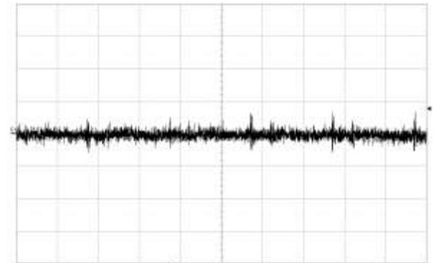
Output voltage ripple at:  $T_{P1} = +25\text{ °C}$ ,  $V_I = 53\text{ V}$ ,  $I_{O1} = 0\text{ A}$ ,  $I_{O2} = 3.6\text{ A}$ ,  $I_{O3} = 0.15\text{ A}$ , resistive loads.
