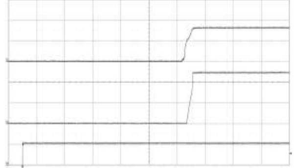
Start-up enabled by connecting  $V_i$  at:  $T_{P1} = +25\text{ °C}$ ,  $V_i = 53\text{ V}$ ,  $I_{O1} = 0\text{ A}$ ,  $I_{O2} = 3.6\text{ A}$ ,  $I_{O3} = 0.15\text{ A}$ , resistive loads.
