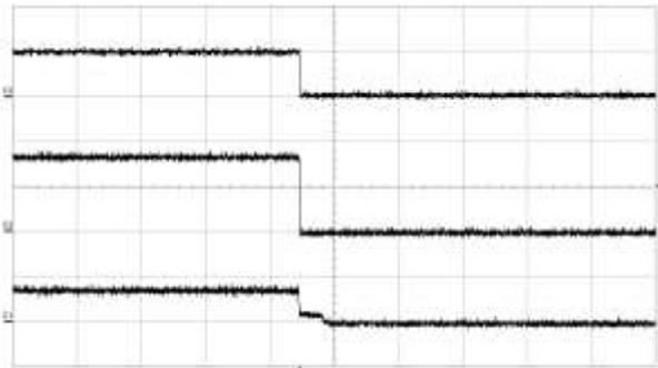
Shut-down enabled by disconnecting  $V_I$  at:  $T_{P1} = +25\text{ °C}$ ,  $V_I = 53\text{ V}$ ,  $I_{O1} = 0\text{ A}$ ,  $I_{O2} = 3.6\text{ A}$ ,  $I_{O3} = 0.15\text{ A}$ , resistive loads.
