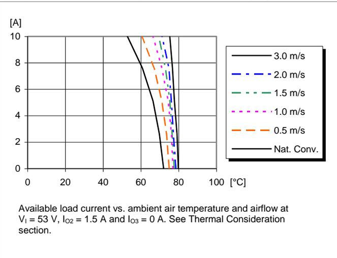
**Output Current Derating, Basic Insulation (PD\*)**
