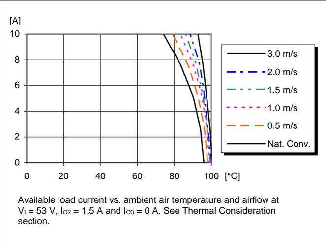
**Output Current Derating, Functional Insulation (PD\*)**
