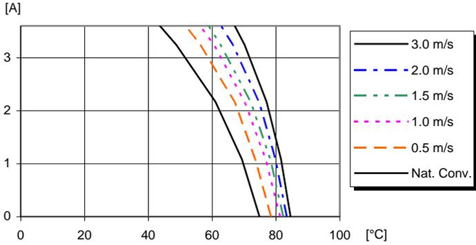
Available load current vs. ambient air temperature and airflow at:
