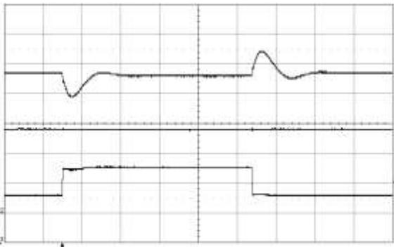
Output voltage response to load current step-change, output 2 (0.9-2.7-0.9 A) at:  $T_{P1} = +25\text{ °C}$ ,  $V_i = 53\text{ V}$ ,  $I_{O1} = 0\text{ A}$ ,  $I_{O3} = 0.15\text{ A}$ , electronic load,  $C_{O2} = 360\text{ }\mu\text{F}$
