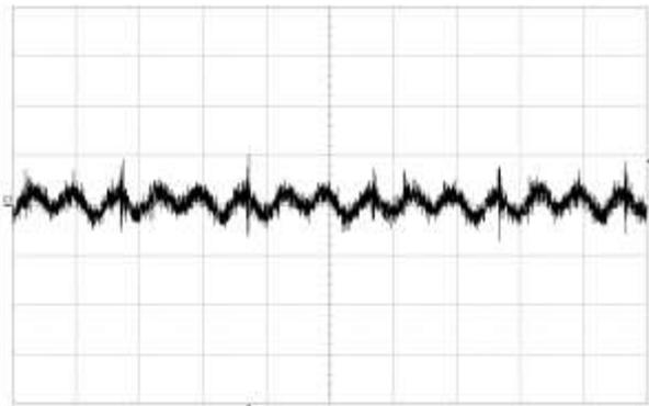
Output voltage ripple at:  $T_{P1} = +25\text{ °C}$ ,  $V_I = 53\text{ V}$ ,  $I_{O1} = 0\text{ A}$ ,  $I_{O2} = 3.6\text{ A}$ ,  $I_{O3} = 0.15\text{ A}$ , resistive loads.
