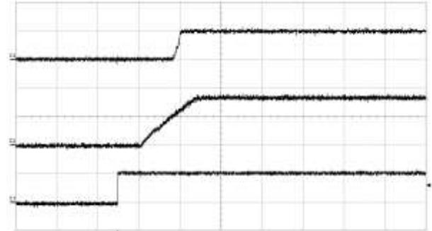
Start-up enabled by connecting  $V_I$  at:  $T_{P1} = +25\text{ °C}$ ,  $V_I = 53\text{ V}$ ,  $I_{O1} = 0\text{ A}$ ,  $I_{O2} = 3.6\text{ A}$ ,  $I_{O3} = 0.15\text{ A}$ , resistive loads.
