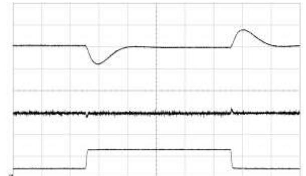
Output voltage response to load current step-change, output 2 (0.9-2.7-0.9 A) at:  $T_{P1} = +25\text{ °C}$ ,  $V_I = 53\text{ V}$ ,  $I_{O1} = 0\text{ A}$ ,  $I_{O3} = 0.15\text{ A}$ , resistive load,  $C_{O2} = 360\text{ μF}$
