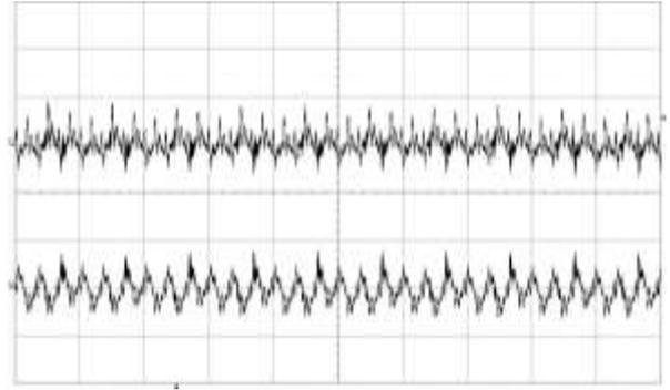
Output voltage ripple at:  $T_{P1} = +25\text{ °C}$ ,  $V_i = 53\text{ V}$ ,  $I_{O1} = 0\text{ A}$ ,  $I_{O2} = 3.6\text{ A}$ ,  $I_{O3} = 0.15\text{ A}$ , resistive loads.
