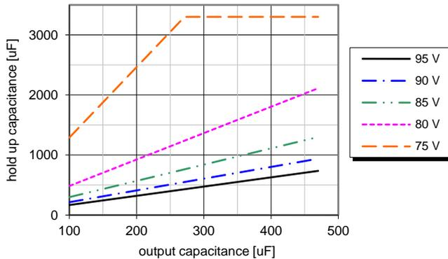
The chart shows output- and hold up capacitances at different hold up voltages for maximum 72 V peak input voltage to the downstream DC/DC converter.
