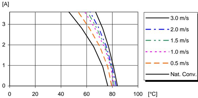
Available load current vs. ambient air temperature and airflow at  $V_I = 53\text{ V}$ ,  $I_{O1} = 4\text{ A}$  and  $I_{O3} = 0\text{ A}$ . See Thermal Consideration section.
