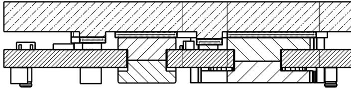
View above showing the milled protrusion for the fets and the 1 mm gappads (see hatch explanation in right info box).
