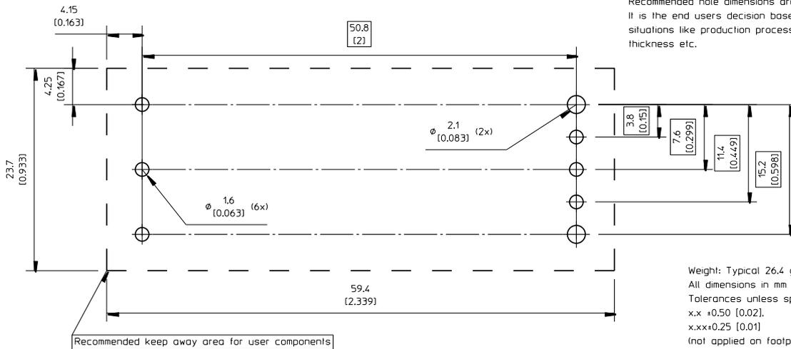
Recommended hole dimensions are only for reference. It is the end users decision based on different situations like production processes, substrate thickness etc.
