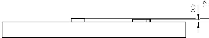
Dimensions for the two protrusions of the cold-wall dimensioned in relation to origo from top-view.
