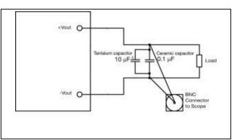
Output ripple and noise test setup
