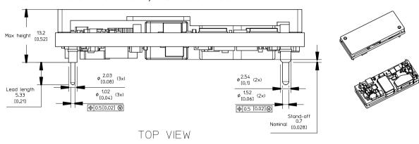
Pin positions according to recommended footprint
