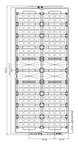
JEDEC standard tray for 2x10 = 20 products. All dimensions in mm [inch] Tolerances:  $X.x \pm 0.26$  [0.01],  $X.xx \pm 0.13$  [0.005] Note: pick up positions refer to center of pocket. See mechanical drawing for exact location on product.
