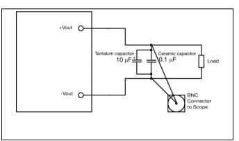
Output ripple and noise test setup
