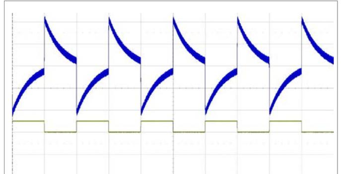
Output voltage response to load current step-change (10-15-10 A) at:
