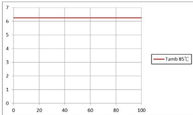
Available load current vs. cold wall temperature.  $V_1 = 110$  V. See Thermal Consideration section.
