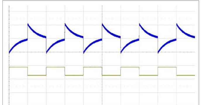
Output voltage response to load current step-change (12.5-18.75-12.5 A) at:
