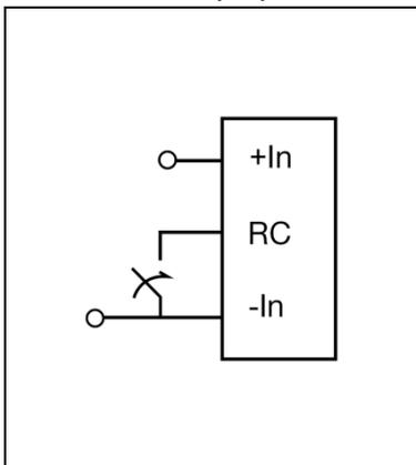
The products are fitted with a remote control function referenced to the primary negative input connection (-In), with negative and positive logic options available. The RC function allows the product to be turned on/off by an external device like a semiconductor or mechanical switch. The RC pin has an internal pull up resistor to +In.
