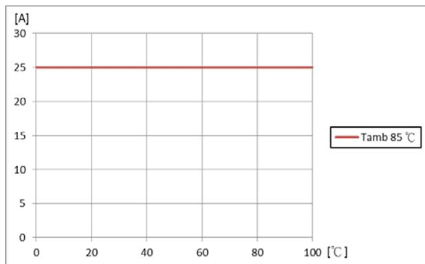
Available load current vs. cold wall temperature.  $V_i = 110$  V.
