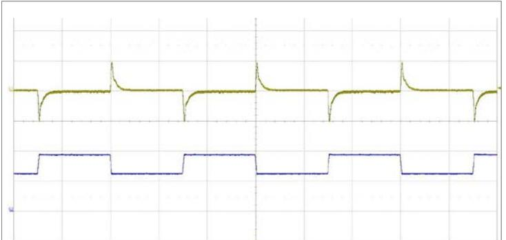
Output voltage response to load current step-change
