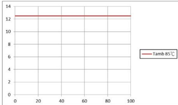
Available load current vs. cold wall temperature.  $V_I = 110$  V. See Thermal Consideration section.
