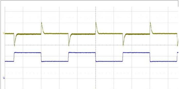
Output voltage response to load current step-change
