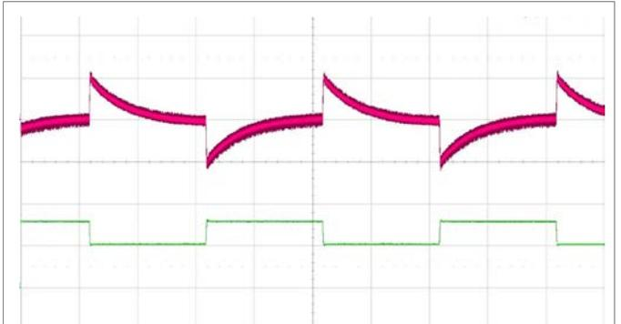
Output voltage response to load current step-change (10.85-16.275-10.85 A) at:
