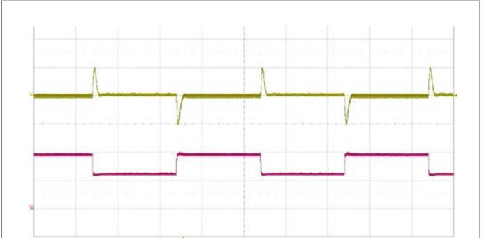
Output voltage response to load current step-change (2.775-4.1625-2.775 A) at:
