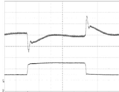
Output voltage response to load current step-change (10-30-10 A) at:
