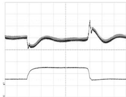
Output voltage response to load current step-change (25-75-25 A) at:
