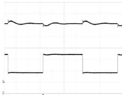
Output voltage response to load current step-
