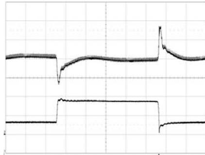
Output voltage response to load current step-change (12.5-37.5-12.5 A) at:
