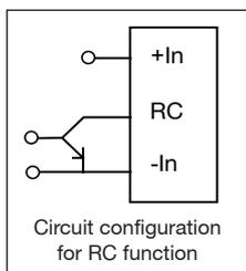
The PKM 4000E Series DC/DC converters have a remote control function referenced to the primary side (- In), with negative and positive logic options available. The RC function allows the converter to be turned on/off by an external device like a semiconductor or mechanical switch. The RC pin has an internal
