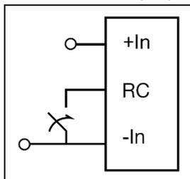
The products are fitted with a remote control function referenced to the primary negative input connection (-In), with negative and positive logic options available. The RC function allows the product to be turned on/off by an external device like a semiconductor or mechanical switch.
