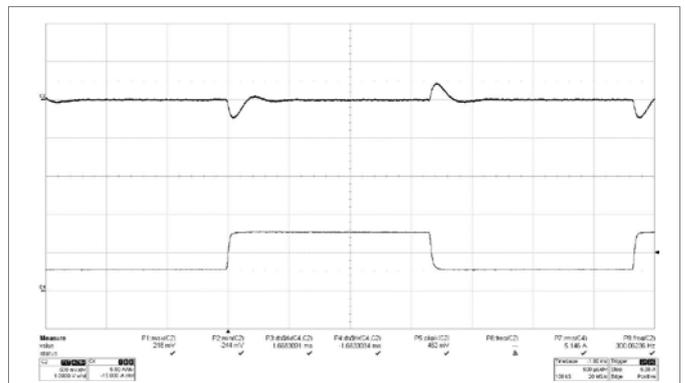
Output voltage response to load current step-
