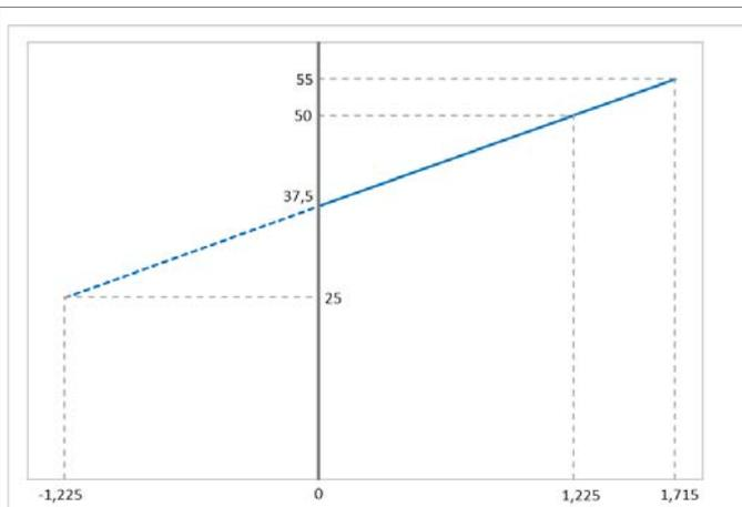
Desired output voltage vs. adjust voltage,  $R_{adj} = 2 \text{ k}\Omega$
