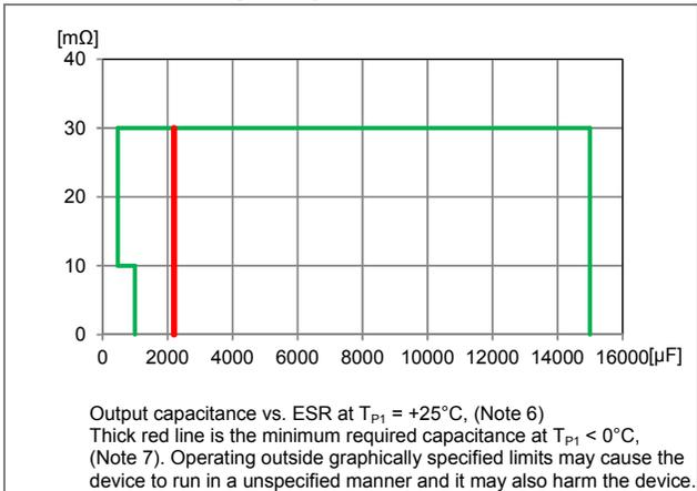
Note 6: ESR include conductor resistance between capacitor and output pins of the device.
