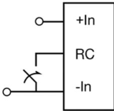
The products are fitted with a remote control function referenced to the primary negative input connection (-In), with negative and positive logic options available. The RC function allows the product to be turned on/off by an external device like a semiconductor, or a mechanical switch placed close to the product. The RC pin has an internal pull up resistor of 10 k $\Omega$  to +5 V. The threshold level has a hysteresis and the function is designed to be robust to noise.
