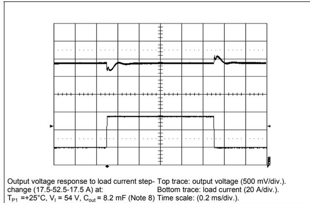
Output voltage response to load current step- change (17.5-52.5-17.5 A) at:
