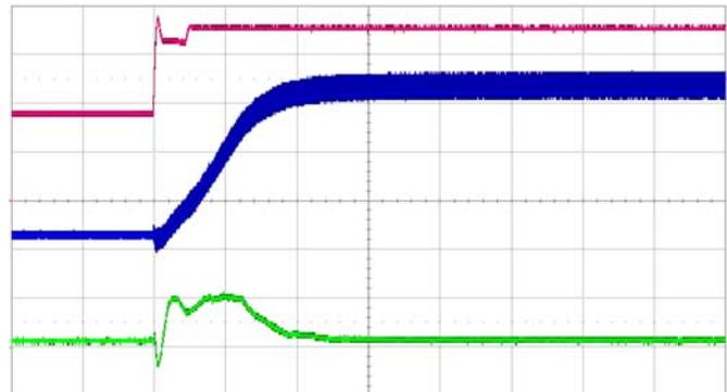
HRR product output at input transient voltage step 36-72 V, 1 ms/div
