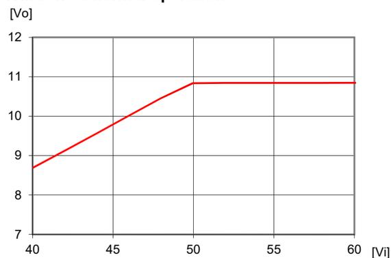
Between 50 and 60 Vin the product operates just like a normally regulated product. It handles load and line transients well and keeps a constant output voltage as well as a constant maximum power.
