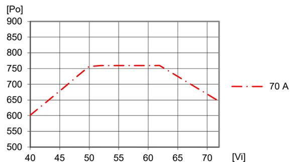
To enable a high power capability at low input voltages the input under voltage lockout is set to start the product when the input voltage reaches the typical value found in the Electrical Specification.
