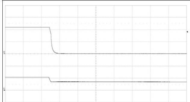
Shut-down enabled by disconnecting  $V_i$  at:
