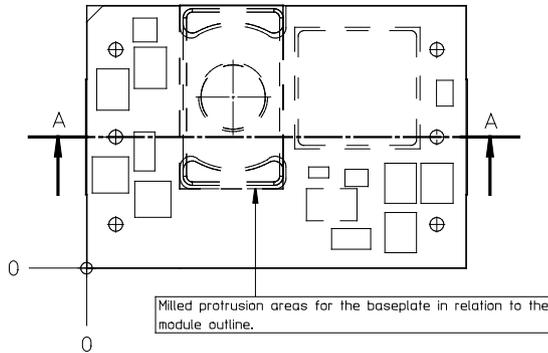
View to the left shows module from top through the coldwall showing the two areas that needs to be milled to meet the FETs for optimal heat evacuation.
