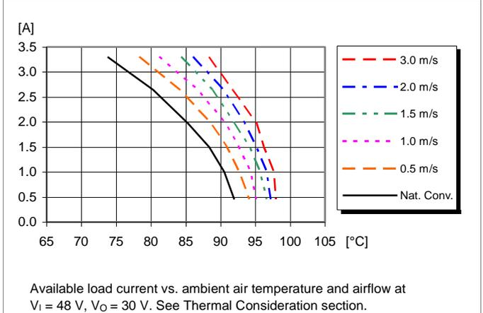
**Output Current Derating – Cold wall sealed box**
