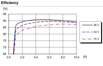
Efficiency vs. load current and input voltage at  $T_{P1}$  = +25°C.
