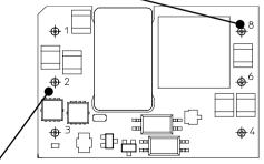
Pin 2 for measurement of maximum product temperature, T<sub>PRODUCT</sub>
