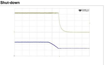
Shut-down enabled by disconnecting V<sub>I</sub> at:  $T_{P1} = +25^{\circ}C$ , V<sub>I</sub> = 53 V,  $I_{O} = 10$  A resistive load.
