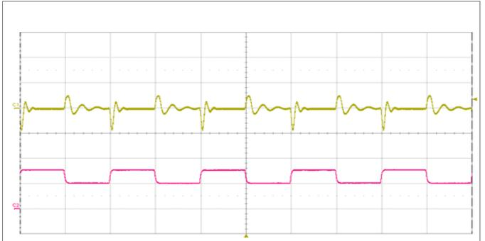
Output voltage response to load current step-
