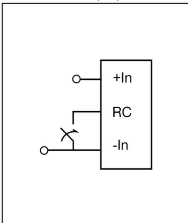
The products are fitted with a remote control function referenced to the primary negative input connection (-In), with negative and positive logic options available. The RC function allows the product to be turned on/off by an external device like a semiconductor or mechanical switch. The RC pin has an internal pull up resistor to +5 V.
