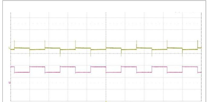
Output voltage response to load current step-change (5.0-7.5-5.0 A) at:
