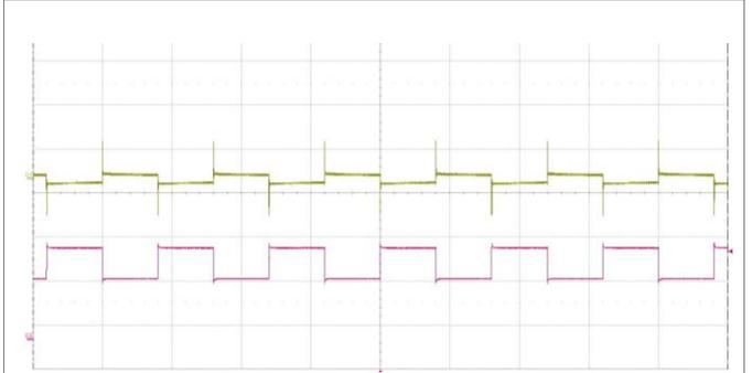
Output voltage response to load current step-change (7.5-11.25-7.5 A) at:
