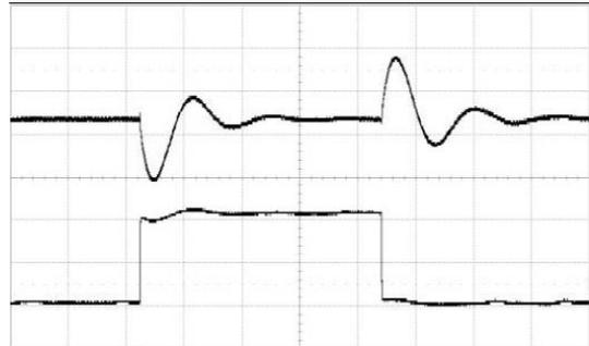
Output voltage response to load current step-change (2.1-6.4-2.1A) at:
