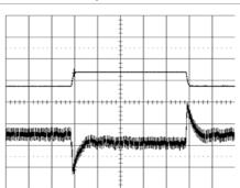
Output voltage response to load current step- Top trace: output voltage (50mV/div.). change (6-12-6 A) at: Bottom trace: load current (10 A/div.).  $T_{ref} = +25^{\circ}C, \ V_{l} = 12.0 \ V.$  Time scale: 0.1 ms/div.
