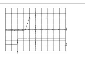
Top trace: output voltage (2.0 V/div.). Bottom trace: input voltage (10 V/div.). Time scale: 10 ms/div.
