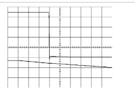
Shut-down enabled by disconnecting  $V_{l}$  at:  $T_{ref}$  = +25°C,  $I_{O}$  = 12 A resistive load,  $V_{l}$  = 12.0 V.
