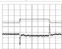
Output voltage response to load current step- Top trace: output voltage (50mV/div.). change (6-12-6 A) at: Bottom trace: load current (10 A/div.).  $T_{ref} = +25^{\circ}\text{C}, \ V_{l} = 12.0 \text{ V}.$  Time scale: 0.1 ms/div.
