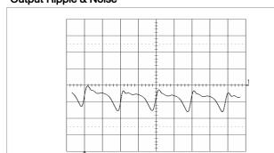
Output voltage ripple (20mV/div.) at:  $T_{ref}$  = +25°C,  $I_O$  = 12 A resistive load,  $V_I$  = 12.0 V. Time scale: 2 µs/div.
