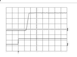
Top trace: output voltage (1.0 V/div.). Bottom trace: input voltage (10 V/div.). Time scale: 10 ms/div.
