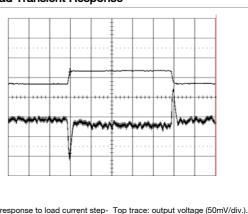
Output voltage response to load current step- Top trace: output voltage (50mV/div.). change (6-12-6 A) at: Bottom trace: load current (10 A/div.).  $T_{ref} = +25^{\circ}C, \ V_{l} = 12.0 \ V.$  Time scale: 0.1 ms/div.
