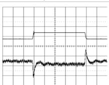
Output voltage response to load current step-change (6-12-6 A) at: Bottom trace: load current (10 A/div.).  $T_{ref} = +25^{\circ}C, \ V_{l} = 12.0 \ V.$  Time scale: 0.1 ms/div.
