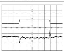
Output voltage response to load current step- Top trace: output voltage (100mV/div.). change (6-12-6 A) at: Bottom trace: load current (5 A/div.).  $T_{ref} = +25^{\circ}\text{C}, \ V_{i} = 12.0 \ \text{V}.$  Time scale: 0.1 ms/div.
