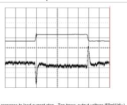
Output voltage response to load current step- Top trace: output voltage (50mV/div.). change (6-12-6 A) at: Bottom trace: load current (10 A/div.).  $T_{ref} = +25^{\circ}C, \ V_{l} = 12.0 \ V.$  Time scale: 0.1 ms/div.
