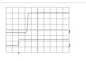
Top trace: output voltage (0.5 V/div.). Bottom trace: input voltage (10 V/div.). Time scale: 10 ms/div.
