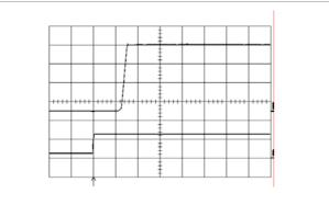
Top trace: output voltage (0.5 V/div.). Bottom trace: input voltage (10 V/div.). Time scale: 10 ms/div.
