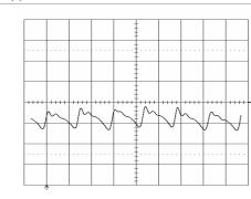
Output voltage ripple (20mV/div.) at:  $T_{ref}$  = +25°C,  $I_O$  = 12 A resistive load,  $V_I$  = 12.0 V. Time scale: 2 µs/div.
