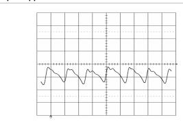
Output voltage ripple (20mV/div.) at:  $T_{ref}$  = +25°C,  $I_O$  = 12 A resistive load,  $V_I$  = 12.0 V. Time scale: 2 µs/div.
