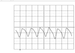
Output voltage ripple (20mV/div.) at:  $T_{ref}$  = +25°C,  $I_O$  = 12 A resistive load,  $V_I$  = 12.0 V. Time scale: 2 µs/div.
