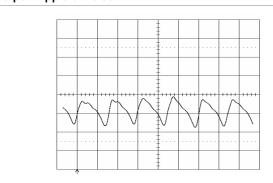
Output voltage ripple (20mV/div.) at:  $T_{ref} = +25^{\circ}C$ ,  $I_{O} = 12$  A resistive load,  $V_{I} = 12.0$  V. Time scale: 2  $\mu$ s/div
