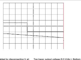
Shut-down enabled by disconnecting V<sub>i</sub> at:  $T_{ref}$  = +25°C, I<sub>O</sub> = 12 A resistive load, V<sub>i</sub> = 12.0 V.
