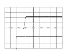
Start-up enabled by connecting V<sub>I</sub> at:  $T_{ref} = +25^{\circ}C$ ,  $I_{O} = 12$  A resistive load,  $V_{I} = 12.0$  V.
