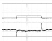
Output voltage response to load current step- Top trace: output voltage (50mV/div.). change (6-12-6 A) at: Bottom trace: load current (10 A/div.).  $T_{ref} = +25^{\circ}C, \ V_{i} = 12.0 \ V.$  Time scale: 0.1 ms/div.
