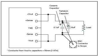
Output ripple and noise test setup
