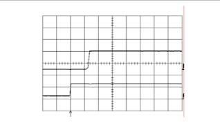
Top trace: output voltage (0.5 V/div.). Bottom trace: input voltage (10 V/div.). Time scale: 10 ms/div.
