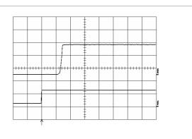
Top trace: output voltage (0.5 V/div.). Bottom trace: input voltage (10 V/div.). Time scale: 10 ms/div.
