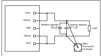
Output ripple and noise test setup
