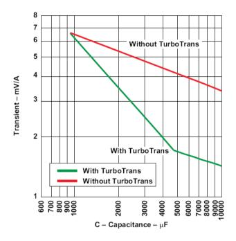
Figure 8. Capacitor Type C, 5000 < C( $\mu$ F)×ESR(mΩ) ≤ 10,000(e.g. OS-CON)
