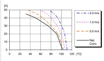
Available load current vs. ambient air temperature and airflow at  $V_1$  = 12 V. See Thermal Consideration section.
