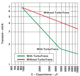
Figure 7. Capacitor Type B, 1000 < C(µF)×ESR(m $\Omega$ ) ≤ 5000 (e.g. Polymer-Tantalum)
