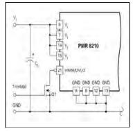
The products are fitted with a remote control function by using the Inhibit/UVLO pin. The Inhibit control function allows the product to be turned on/off by an external device like a semiconductor or mechanical switch. The RC pin has an internal pull up. An external pull-up resistor should never be used with the inhibit pin.
