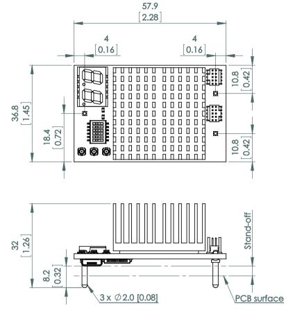
Weight: Typical 54g All dimensions in mm [inch] Tolerances unless specified ±0.25 [0.01]
