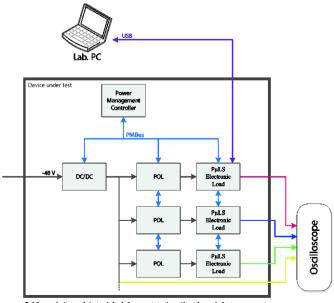
PµLS can substitute real electronic loads for accurate testing without the need of extra components
