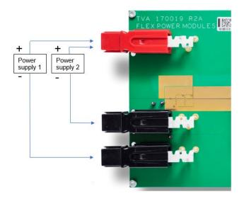
Picture 3: Connection of power supplies for input voltage transient testing
