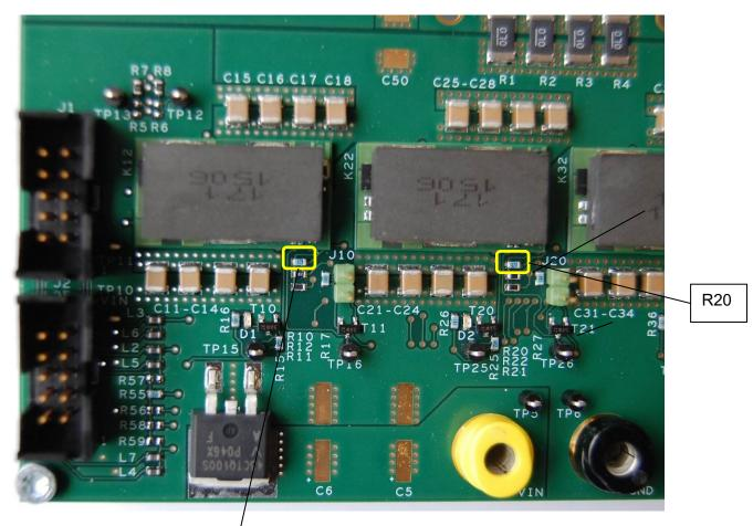
Figure 5.1/Vset resistors for 2 of 4 module positions are shown in the picture.
