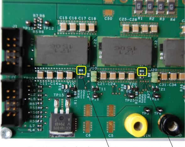
Fig 5.2 Address resistors for 2 of 4 module positions are shown in the picture.
