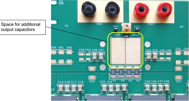
Fig 7 Space for additional output capacitors.
