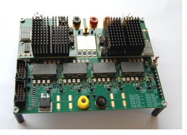
Fig 8 Puls loads connected to the board.
