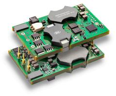
BMR 457 SERIES 25 A Digitally controlled 3E Isolated DC/DC Advanced Bus Converter (Isolated DC/DC Converter) Efficiency, typ. 95.5% Input voltage range, 36-75 V Output power 300 W Size (LxWxH): 58.4 x 22.7 x 10.2 mm (2.30 x 0.89 x 0.40 inch)
