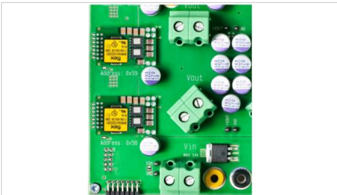
Figure 19: PoL parallel test board setup for this example—two BMR463 modules at addresses 0x58 and 0x59
