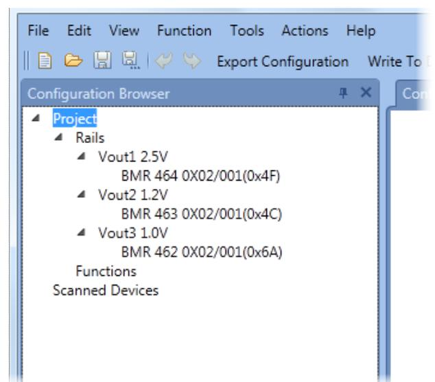
Figure 11. Rails for Example 3 in Flex Power Designer. Without any sequencing added yet, this is the same Rail setup as in Example 1
