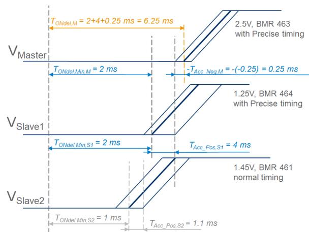
Figure A5. TON\_DELAY calculations for tracking master using Eq. A2.
