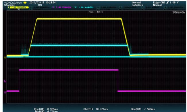
Figure 22 Coincident Tracking – Power-on/off sequence of a BMR 464 as tracking master (TON\_DELAY = 10ms, TOFF\_DELAY = 0ms, Vout = 3.,3V in yellow color) and a BMR 465 as tracking slave (TON\_DELAY = 0 ms, TOFF\_DELAY = 35ms, Vout = 1V in light blue color) CTRL signal is shown in lilac color. The oscilloscope plot shows 100 accumulated tests. ( x-scale is 20 ms/div).
