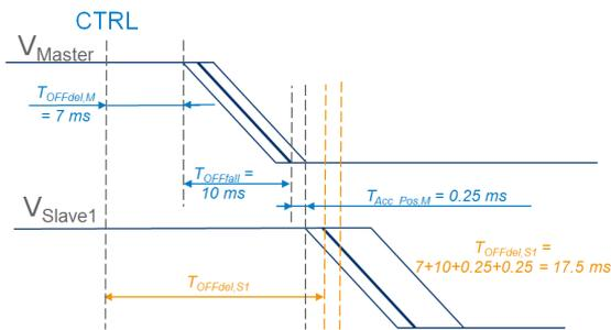
Figure A6. TOFF\_DELAY calculations for the two tracking slaves using Eq. A4.
