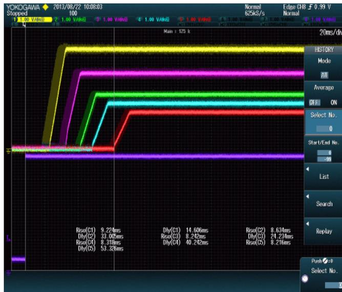
Figure A8. Time-based up-sequencing accumulated variations from 100 power-up occasions, without precise timing of BMR 462-464 room temperature. The CTRL signal, the bottom trace, triggers the start of all five rails. As seen, the accuracy of the start-up time for each rail is in the range of {-0.25, 4ms} related to the CTRL signal positive ramp. Note: The 1.5V rail (in light blue color), is configured for precise-timing ramp-up. (20 ms/div).
