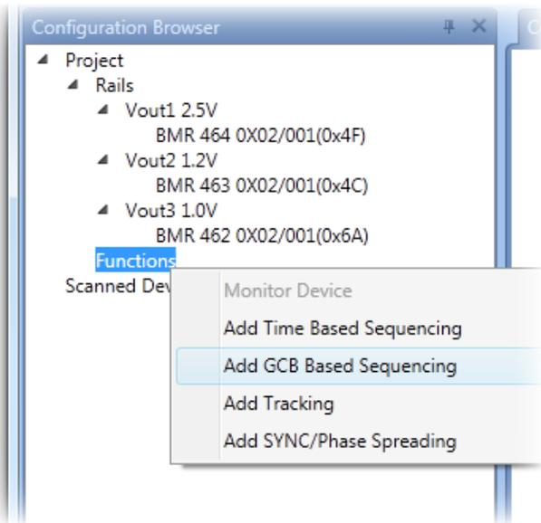
Figure 12. Adding GCB Based Sequencing
