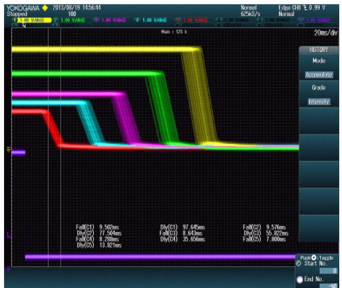
Figure A17. GCB-based down-sequencing accumulated variations from 100 power-down occasions of BMR 462-464. The CTRL signal, the bottom trace, triggers the start of all five rails. The configured total down-sequencing time, incl timing variation, is 105.0 – 118.0 ms. This is due to the fact that the timing error in previous rails are accumulated. However, non-overlap is always granted in GCB-based sequencing. (20 ms/div).
