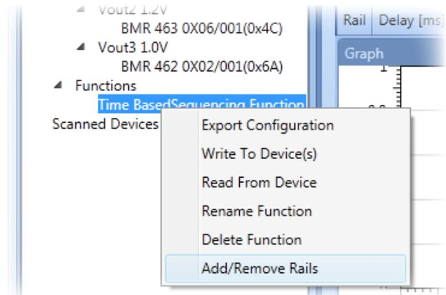
Figure 5. Adding Rails to the Sequencing Function.
