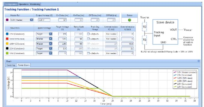
Figure A19. Voltage tracking power-down configuration of 6 rails using Flex Power Designer design tool.
