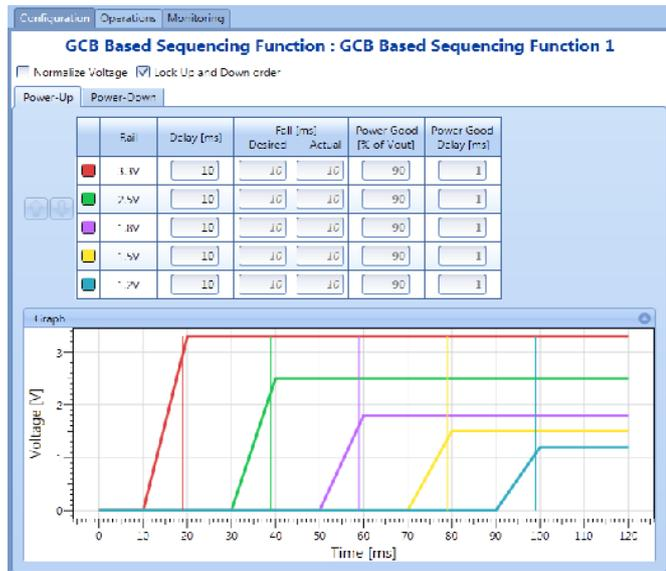
Figure A14. GCB-based power-up sequencing configuration of 5 rails using Flex Power Designer design tool. The total configured power-up time until last rail's PG is asserted is 98 ms.
