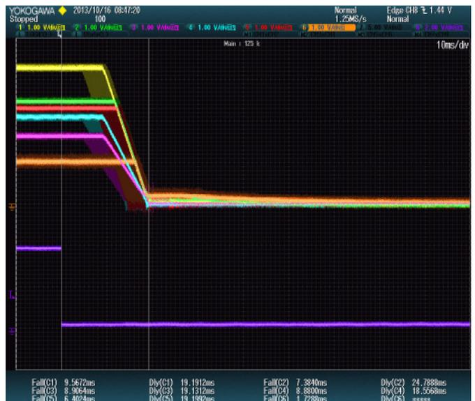
Figure A21. Voltage down-tracking accumulated variations from 100 power-down occasions. The CTRL signal, the bottom trace, triggers the start of the tracking master rail. Compared to power-up, the timing variation between different start-up occasions is quite large. Still the tracking slaves follows the tracking master closely in each start-up occasion. This is however not possible to see in this plot. The statistics are collected in Table A1. (20 ms/div).
