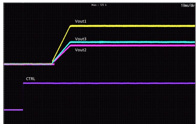
Figure 21 Tracking – Turn-on sequence example. (x-scale is 10 ms/div)
