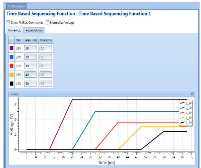
Figure A7. Time-based power-up sequencing configuration of 5 rails using Flex Power Designer design tool. The configured time space between the rails is 10ms.
