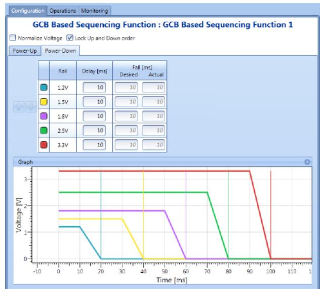
Figure A15. GCB-based power-down sequencing configuration of 5 rails using Flex Power Designer design tool. Total configured power-down time until last rail starts to fall is 90 ms.
