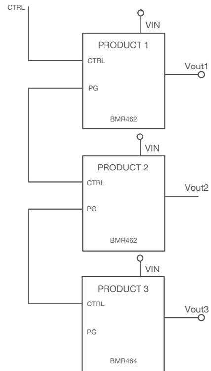
Figure 8 Event based sequencing example. A change of sequencing order will require a hardware re-configuration.
