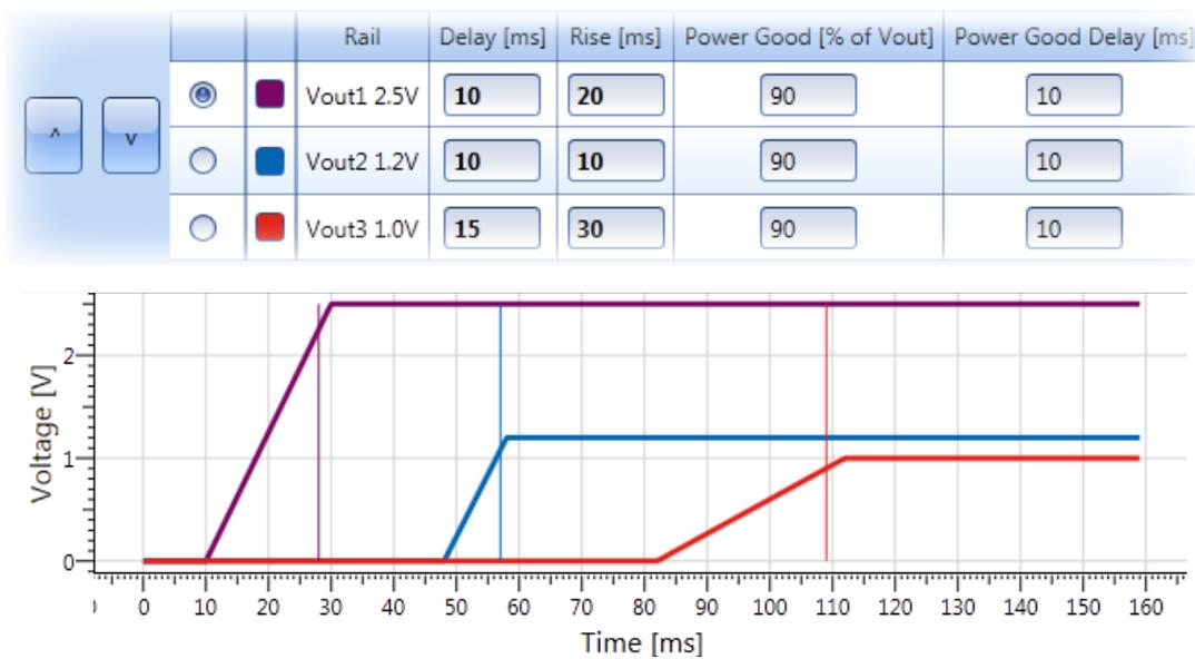
Figure 14a. GCB Based Power-Up Sequencing. There arrow buttons allow one to change the sequencing order.
