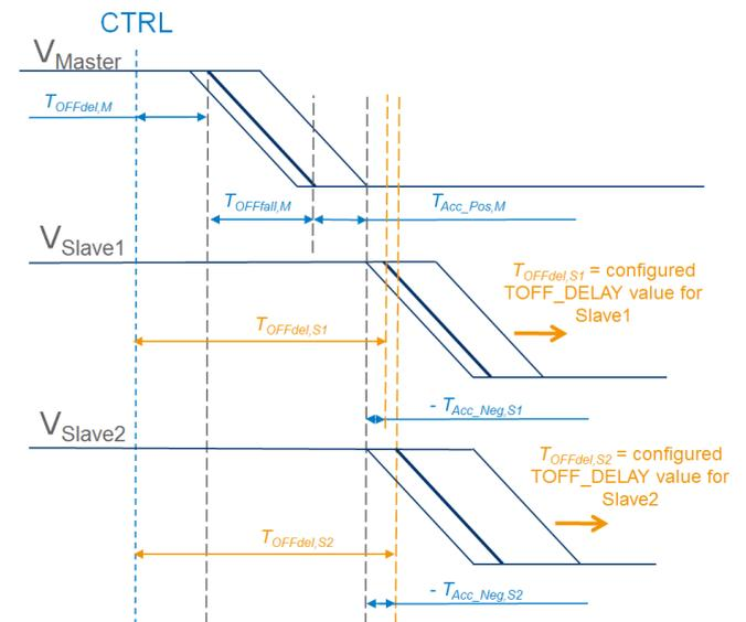
Figure A2. Calculation of smallest possible turn-off delay values of the slaves using Eq. A4.
