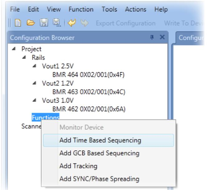
Figure 4. Adding Time Based Sequencing.
