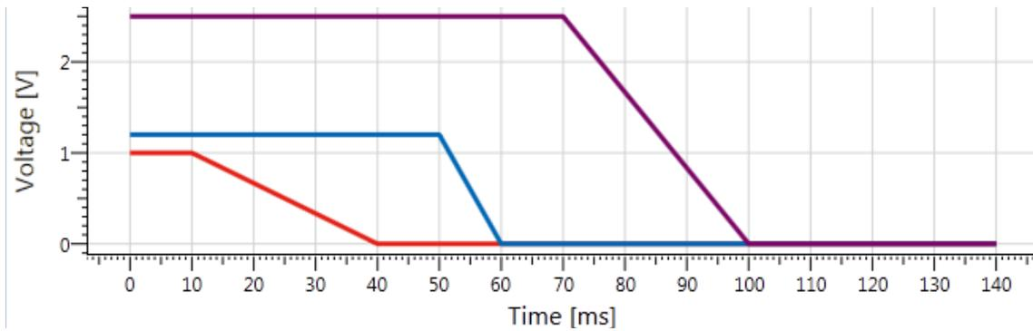
Figure 14b. GCB Based Power-Up Sequencing. There arrow buttons allow one to change the sequencing order.
