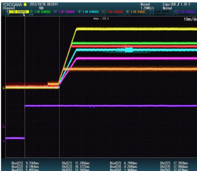
Figure A20. Voltage up-tracking accumulated variations from 100 power-up occasions. The CTRL signal, the bottom trace, triggers the start of the tracking master rail. The tracking master, a BMR 463 0002/001 (3.3V) is configured with precise-ramp-up timing. As seen, the tracking slaves are following the master closely and the timing variation is small. The statistics are collected in Table A1. (20 ms/div).
