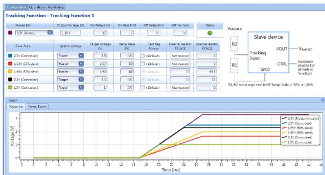
Figure A18. Voltage tracking power-up configuration of 6 rails using Flex Power Designer design tool.
