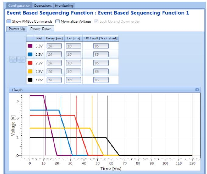
Figure A11. Event-based power-down sequencing configuration of 5 rails using Flex Power Designer design tool. The configured shut-down time for all rails is 66 ms.
