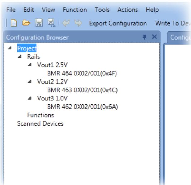
Figure 3. Rails from Example 1 in Flex Power Designer.
