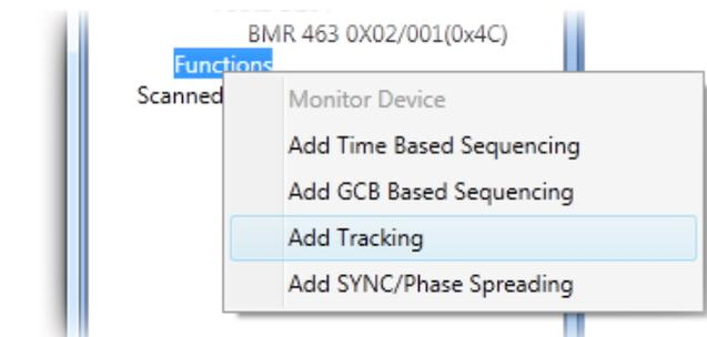
Figure 17 Adding Voltage Tracking Function.
