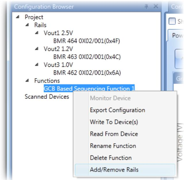
Figure 13. Adding GCB Based Sequencing
