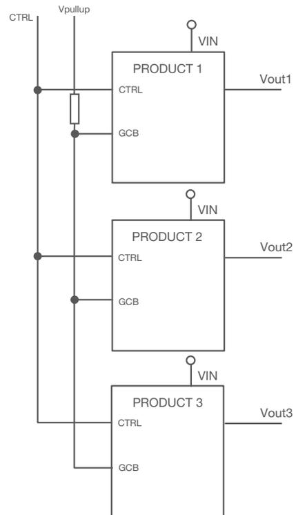
Figure 10 GCB Based Sequencing example – Enabling is shown generated via CTRL pin, but can also be done without a common CTRL by using PMBus OPERATION command.
