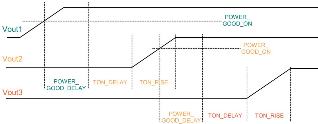
Fig 9a GCB and Event based up-sequencing – Illustration of which settings to be made in which rail. The total time between the Preceding rail, Vout1, and the following rail, Vout2, is determined as follows: Vout1 is configured using POWER\_GOOD\_ON and POWER\_GOOD\_DELAY while Vout2 is configured using TON\_DELAY and TON\_RISE
