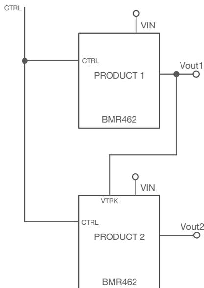
Figure 16 Voltage Tracking Configuration.
