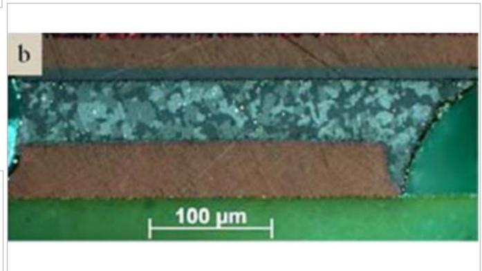
Picture 4: Cross polarized image of a 30 mil SAC305 LGA solder joint exhibiting an interlaced twinned grain structure
