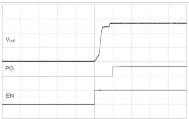
Output enabled by EN pin. V_{in} = 54\text{ V} , I_{out} = 1\text{ A} Scale from top: 5, 5, 5 V/div, 10 ms/div.
