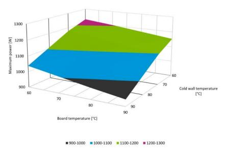
Max average output current vs. cold plate temperature (x-axis) and host board temperature. Thermal interface gap pad 1.0 mm, 8 W/mK.
