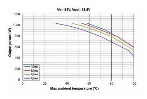
Max avreage output power vs. ambient temperature Thermal interface gap pad to heat sink is 1.0 mm, 8 W/mK.
