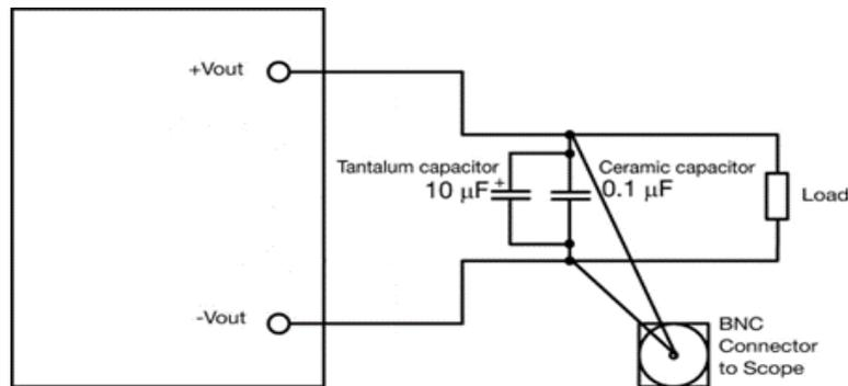
Output ripple and noise test setup
