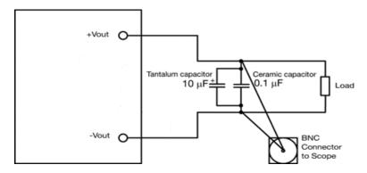
Output ripple and noise test setup
