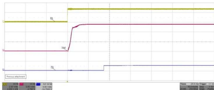
Output disabled by EN pin.  $V_{in} = 54\text{ V}$ ,  $I_{out} = 80\text{ A}$
