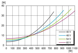
Dissipated power vs. load power at  $T_{P1} = +25$  °C.
