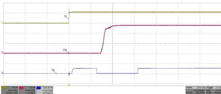
Output enabled by EN pin.  $V_{in} = 54\text{ V}$ ,  $I_{out} = 2\text{ A}$
