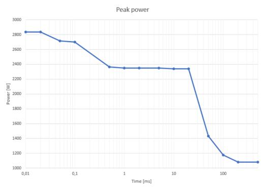
Max peak output current vs pulse duration and PMBus monitored temperature when pulse starts. Input voltage 54V and initial lout = 60 A.
