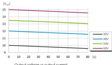
Output voltage vs output current.
