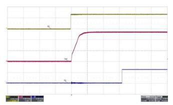
Output enabled by EN pin. Vin = 54 V, Iout = 2 A Scale from top: EN=2, Vout=5, PG pin=2 V/div, 5 ms/div.
