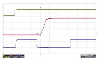
Output enabled by Vin. Vin = 54 V, Iout = 2 A Scale from top: Vin=50, Vout=5, PG pin=2 V/div, 5 ms/div.
