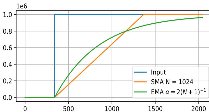
Demonstration of the behaviour of Simple Moving Average (SMA) and EMA for a step-function input
