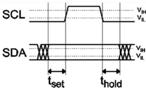
Set-up and hold timing diagram
