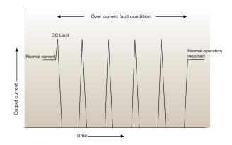
Figure 9 - Example of Over Current Protection with hiccup limiting
