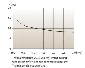
Figure 7 - Example of thermal resistance curve
