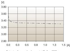
Output voltage vs. load current at Tref =  $+25^{\circ}$ C
