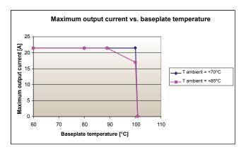
Figure 3 - PKY2616PI Available output current vs. baseplate temperature at  $\rm V_{in}{=}27\,\rm V$
