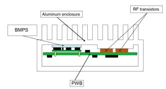
Figure 1 - Sealed box application example
