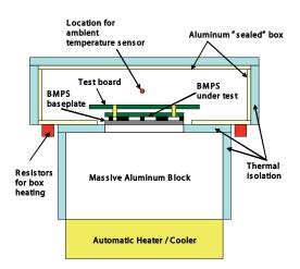
Figure 2 - Cross-section of the test equipment
