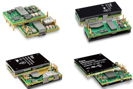
For Microwave applications, lower power solutions of 100W are available in sixteenth brick packages, delivering low power radio-specific output voltages of 5-7V and a wide range of 12V IBC solutions.
