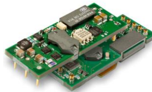
Figure 1 PKB4000A Size LxWxH 58.4x22.7x8.5mm
