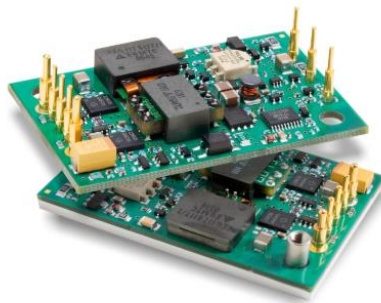
Figure 1 PKM4000E PI QB Size LxWxH 57.9x36.8x8.5mm
