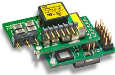
Picture 4 BMR463 product SIP size: 26.3 x 7.6 x 15.6 mm (1.035 x 0.30 x 0.614 in) Laydown size: 25.65 x 13.8 x 8.2 mm (1.01 x 0.543 x 0.323 in)
