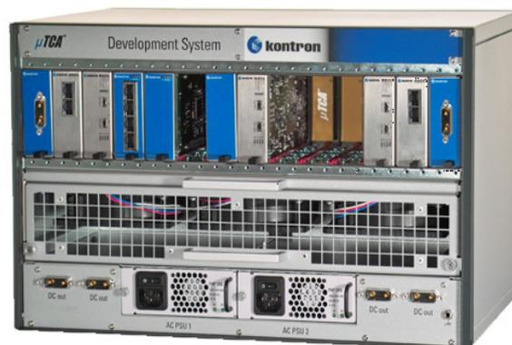
Figure 5 – MicroTCA sub-rack holding AdvancedMCs and power modules
