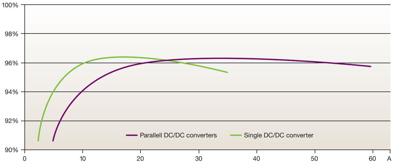
Figure 7 – Efficiency of the paralleled DC/DC converter implementation
