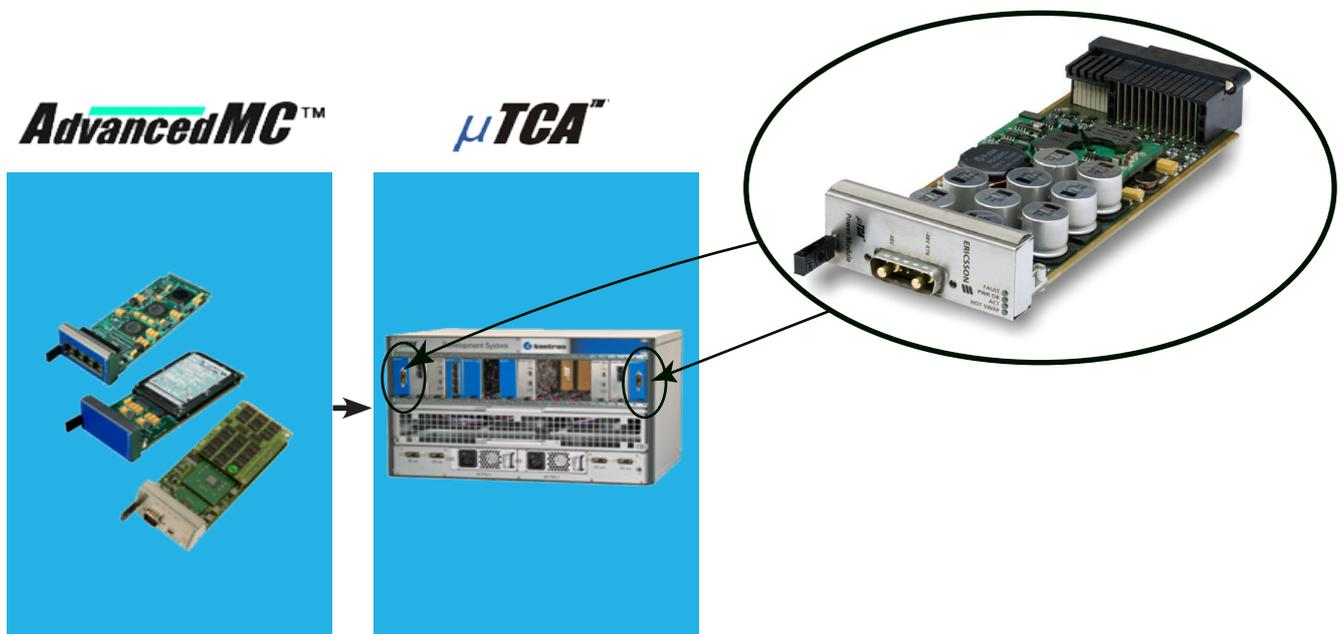
Figure 1 – MicroTCA sub-rack holding AdvancedMCs and power modules
