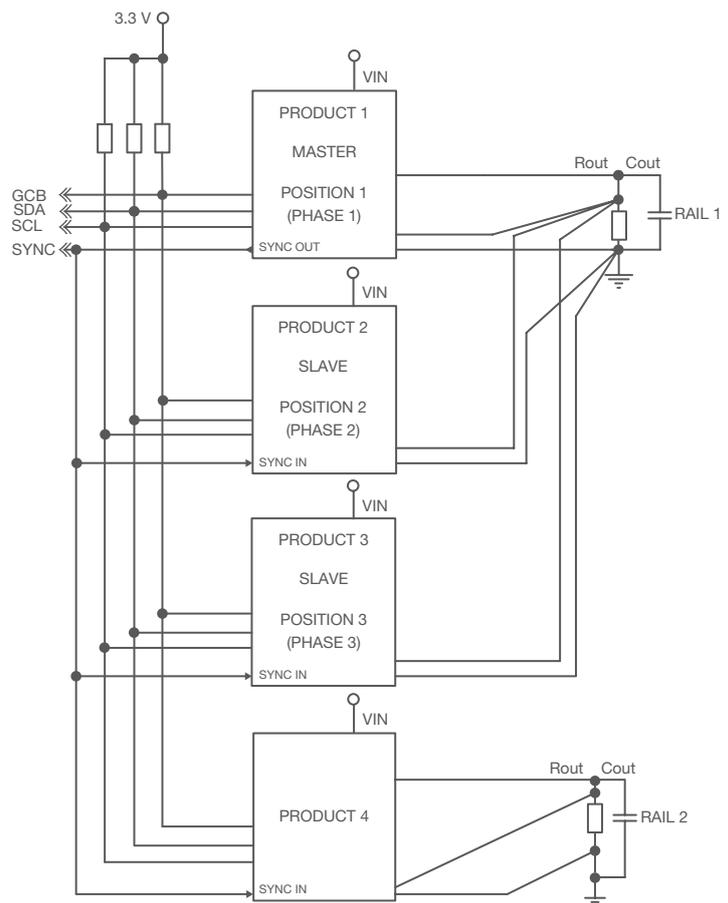
Figure 8. Example of sharing group and auxiliary output rail with a common SYNC clock.
