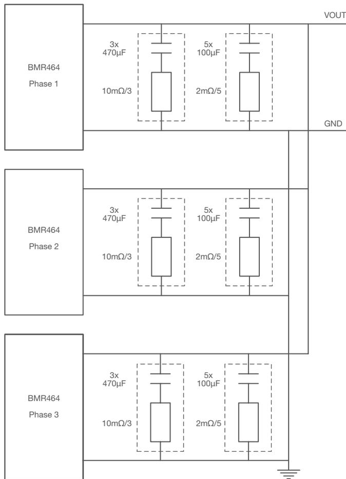
Figure 18. 3-phase current sharing example.
