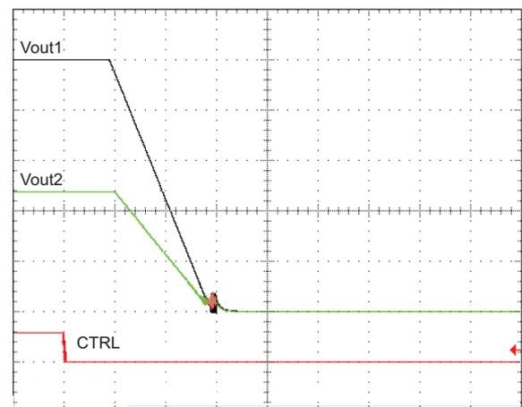
Figure 10 Tracking – Turn-on sequence example.( x-scale is 10 ms/div)
