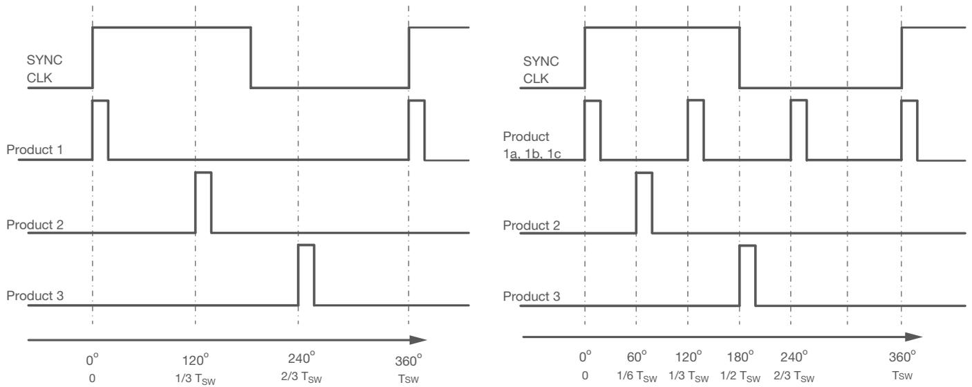
Figure 3. Phase spreading example with three products.
