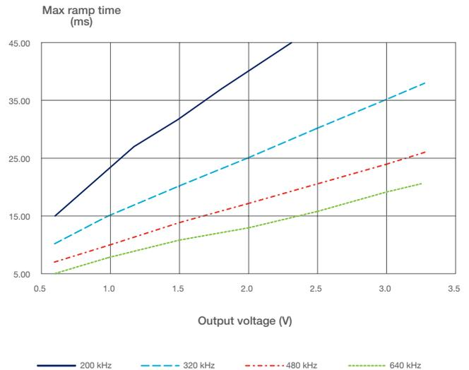
Figure 22. Max ramp time vs output voltage and switch frequency
