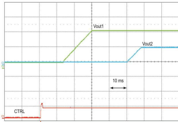
Figure 6a GCB-based sequencing example – Turn-on.
