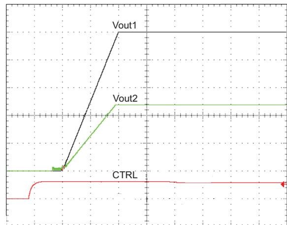
Figure 9 Tracking – Turn-on sequence example.( x-scale is 10 ms/div)
