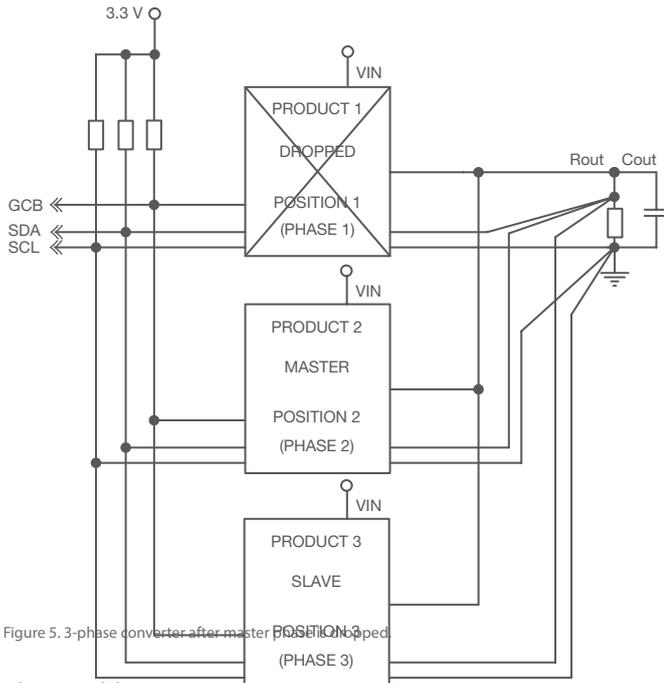
Figure 5. 3-phase converter after master dropped
