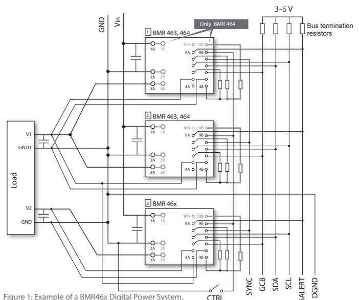
Figure 1: Example of a BMR46x Digital Power System.
