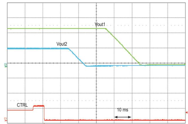
Figure 6b GCB-based sequencing example – Turn-off.
