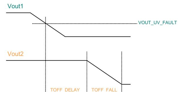
Fig 3b Event based down-sequencing – Illustration of which settings to be made in which rail. The total time between the Preceding rail, Vout1, and the following rail, Vout2, is determined as follows: Vout1 are configured using VOUT\_UV\_FAULT while Vout2 are configured using TOFF\_DELAY and TOFF\_FALL.
