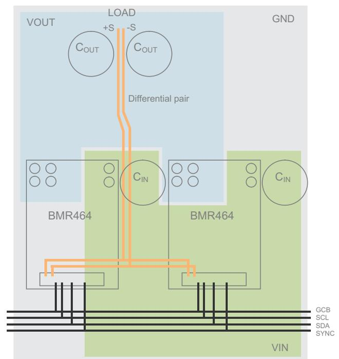
Figure 17. Layout example, two products.
