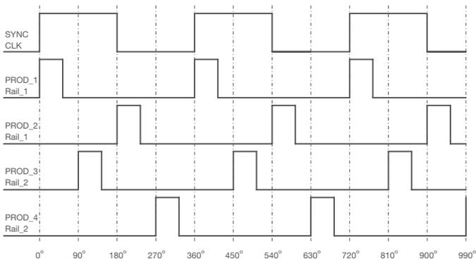
Figure 12. 2 x 2-phase current sharing groups now equally offset using the INTERLEAVE command.
