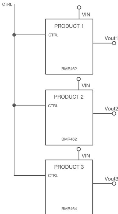
Figure 1. Time based sequencing example.
