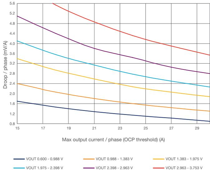
Figure 21. Recommended maximum individual droop per phase vs VOUT and max IOUT for BMR463.
