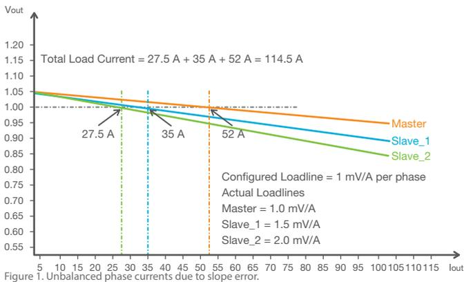
Figure 1. Unbalanced phase currents due to slope error.
