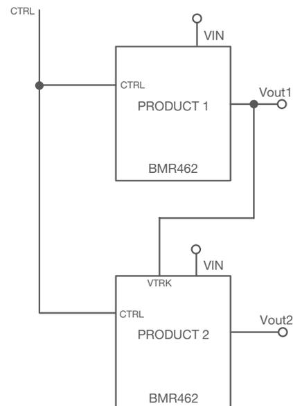
Figure 7 Voltage Tracking Configuration
