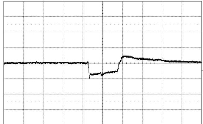
Figure 7. Example of output voltage deviation during drop (10 mV/div, 10 ms/div)
