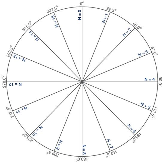
Figure 5. Phase offset resolution wheel.
