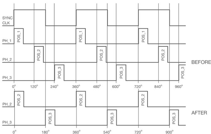
Figure 6. 3-phase converter timing diagram before and after Phase\_1 (Master Phase) is dropped.
