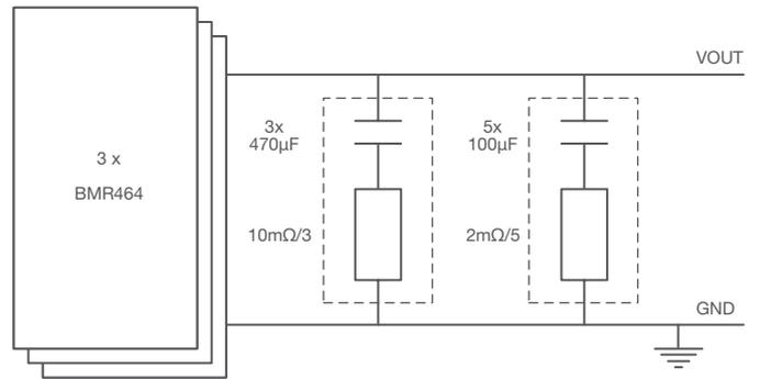
Figure 19. Current sharing compensation model.
