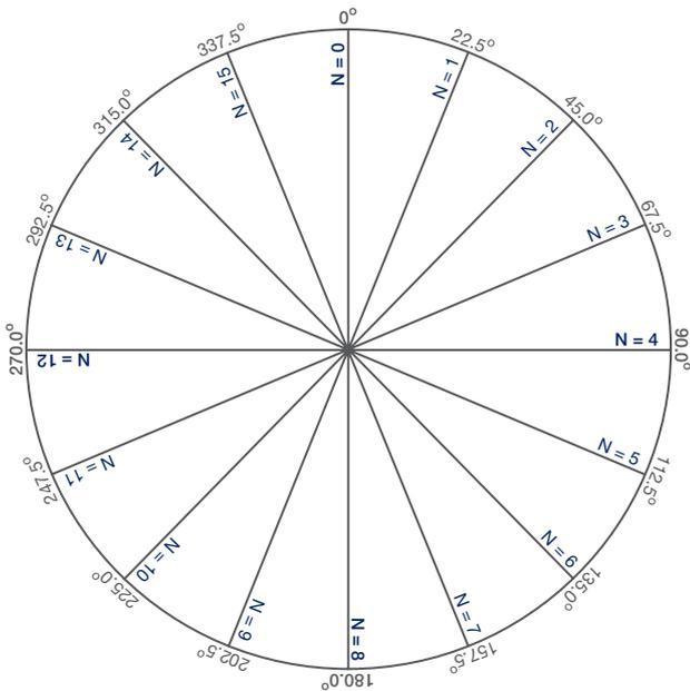
Figure 9. Phase offset resolution wheel.
