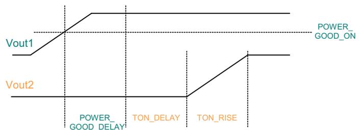
Fig 3a GCB and Event based up-sequencing – Illustration of which settings to be made in which rail. The total time between the Preceding rail, Vout1, and the following rail, Vout2, is determined as follows: Vout1 are configured using POWER\_GOOD\_ON and POWER\_GOOD\_DELAY while Vout2 are configured using TON\_DELAY and TON\_RISE.
