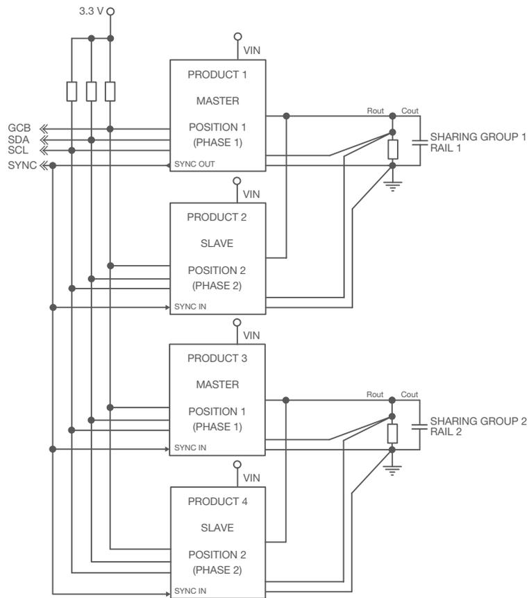
Figure 10. Example of 2 x 2-phase current sharing groups using the same SYNC clock.
