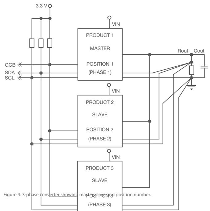
Figure 4. 3-phase converter showing master position and position number.
