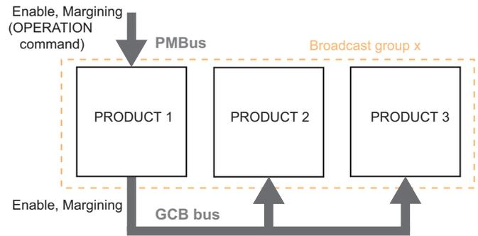
Figure 16. Enable or margining signal will broadcast on the GCB bus.
