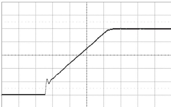
Figure 15. Effect of minimum duty cycle at ramp-up.
