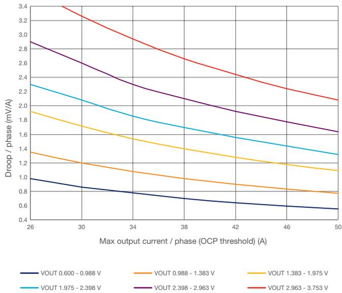
Figure 20. Recommended maximum individual droop per phase vs VOUT and max IOUT for BMR464.
