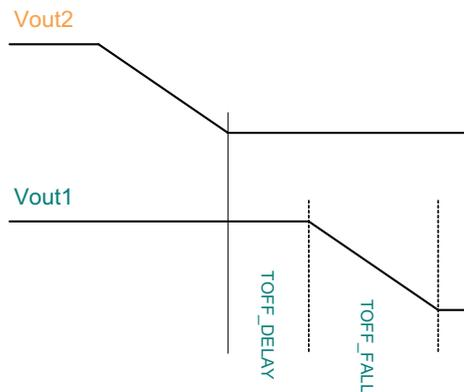
Fig 5 GCB based down-sequencing – Illustration of which settings to be made in which rail. The total time between the Preceding rail, Vout1, and the following rail, Vout2, is determined as follows: When Vout2 has reached 0V, the start of Vout1 triggers. Vout1 are configured using TOFF\_DELAY and TOFF\_FALL.
