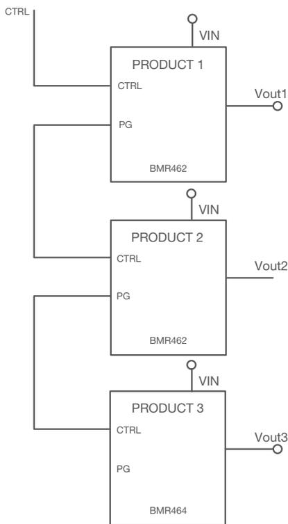
Figure 2 Event based sequencing example. A change of sequencing order will require a hardware re-configuration.
