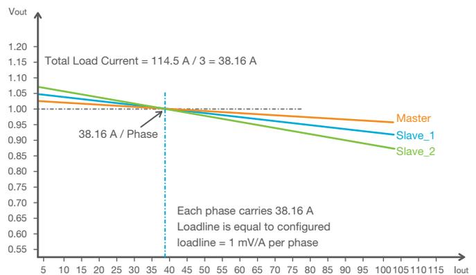
Figure 2. Balanced phase currents. Slave reference voltage(s) is trimmed until all products' currents equalize.
