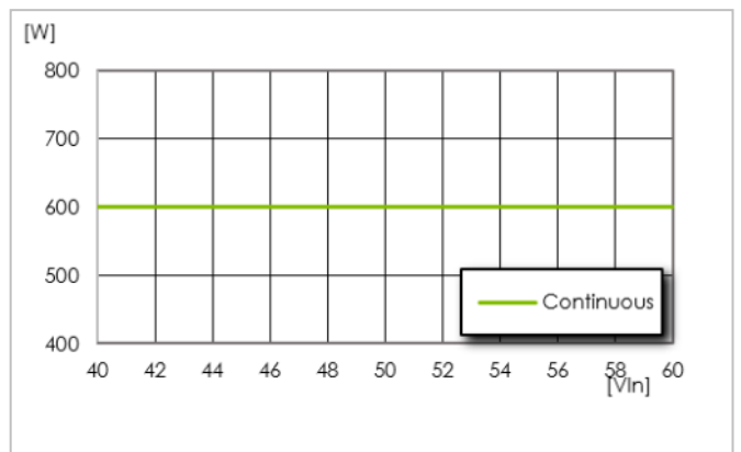
Available output power vs. input voltage, T_{PI} = +90^{\circ}C
