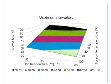
Available output power vs. pin and baseplate temperature See Thermal Consideration section. Above Pout\_TDP, 1300W only for a limited time.
