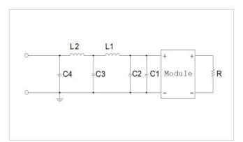
Filter components: C1 = 1000μF (e-lyt) C2 = 2 x 2.2 μF C3, C4 = 10 μF L1, L2 = 4.7 μH
