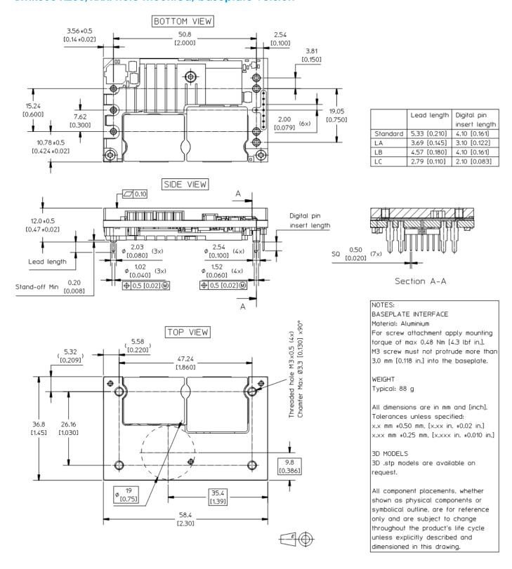
The mechanical information is based on a module which is hole mounted and has a baseplate.
