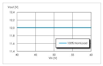
Output voltage vs. input voltage at  $T_{P1}$  = +90°C, 100% of max Pout\_TDP, 1300W.
