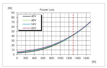
Dissipated power vs. load power at  $T_{P1}$  = +25°C. Above Pout\_TDP, 1300W only peak t  $\leq$  1000ms
