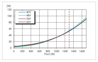
Dissipated power vs. output power and input voltage at  $T_{P1}$  = +90°C, Above Pout\_TDP, 1300W only peak t  $\leq$  1000ms
