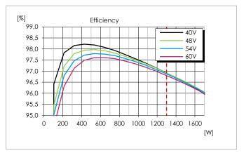
Efficiency vs. output power and input voltage at  $T_{P1}$  = +25°. Above Pout\_TDP, 1300W only peak  $t \le 1000$ ms
