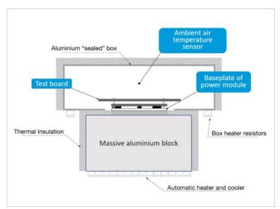
Picture: cold wall test set-up
