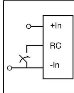
The device should be capable of sinking 0.7 mA. When the RC pin is left open, the voltage generated on the RC pin is max 6 V. The standard product is provided with “negative logic” remote control and will be off until the RC pin is connected to the -In. To turn on the product the voltage between RC pin and -In should be less than 1 V.
