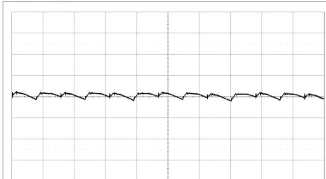
Fundamental output voltage ripple at  $V_i = 12\text{ V}$ ,  $I_o = \text{max } I_o$ ,  $C_{OUT} = 10 \times 470\text{ }\mu\text{F}/5\text{ m}\Omega + 10 \times 100\text{ }\mu\text{F}$ .
