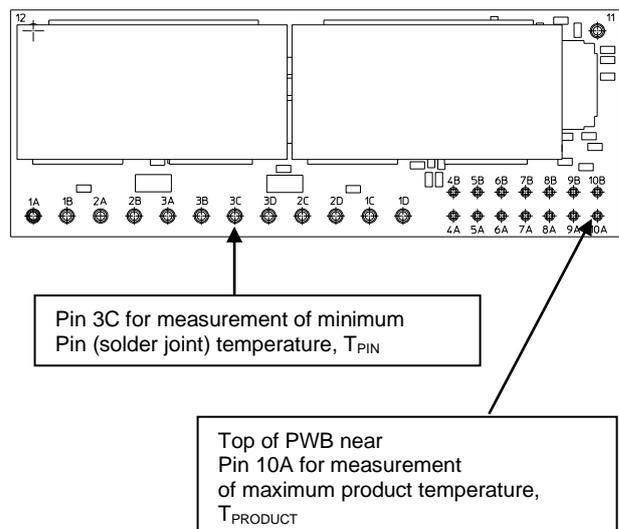
Pin 3C for measurement of minimum Pin (solder joint) temperature,  $T_{PIN}$
