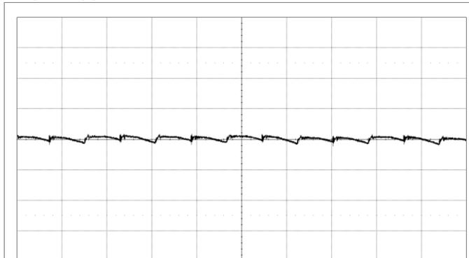
Fundamental output voltage ripple at  $V_I = 12\text{ V}$ ,  $I_O = \text{max } I_O$ ,  $C_{OUT} = 10 \times 470\ \mu\text{F}/5\ \text{m}\Omega + 10 \times 100\ \mu\text{F}$ .
