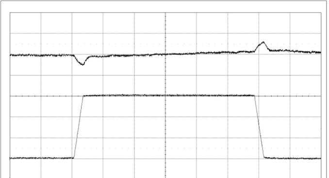
Output voltage response to load current step change (30–90–30 A) at  $V_i = 12\text{ V}$ ,  $C_{OUT} = 10 \times 470\ \mu\text{F}/5\ \text{m}\Omega + 10 \times 100\ \mu\text{F}$ ,  $di/dt = 2\ \text{A}/\mu\text{s}$ , ASCR Gain = 300 and ASCR Residual = 90.
