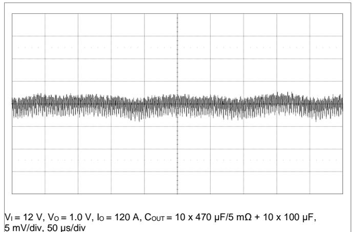
$V_i = 12\text{ V}$ ,  $V_o = 1.0\text{ V}$ ,  $I_o = 120\text{ A}$ ,  $C_{OUT} = 10 \times 470\text{ µF}/5\text{ m}\Omega + 10 \times 100\text{ µF}$ , 5 mV/div, 50 µs/div
