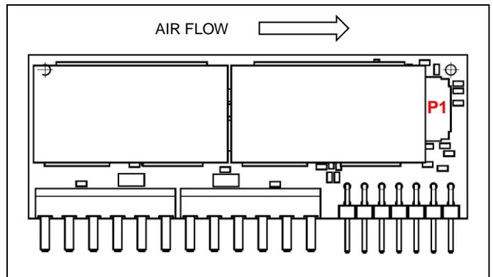
Temperature positions and air flow direction (side view).
