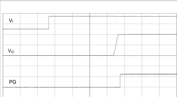
Output enabled by applying  $V_i$ .  $V_i = 12\text{ V}$ ,  $I_o = \text{max } I_o$ .
