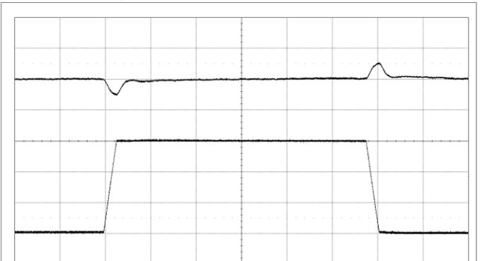
Output voltage response to load current step change (30–90–30 A) at  $V_i = 12\text{ V}$ ,  $C_{OUT} = 10 \times 470\text{ }\mu\text{F}/5\text{ m}\Omega + 10 \times 100\text{ }\mu\text{F}$ ,  $di/dt = 2\text{ A}/\mu\text{s}$ , ASCR Gain = 300 and ASCR Residual = 90.
