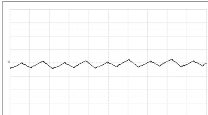
Fundamental output voltage ripple at  $V_I = 12\text{ V}$ ,  $I_O = 60\text{ A}$ ,
