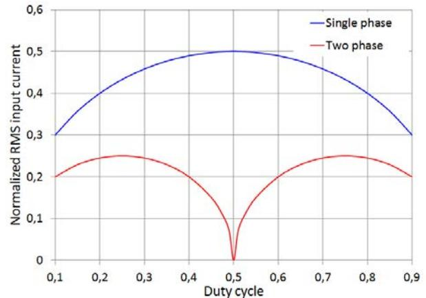
The input ripple RMS current in a buck converter can be estimated to
