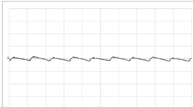
Fundamental output voltage ripple at  $V_I = 12\text{ V}$ ,  $I_O = 80\text{ A}$ ,
