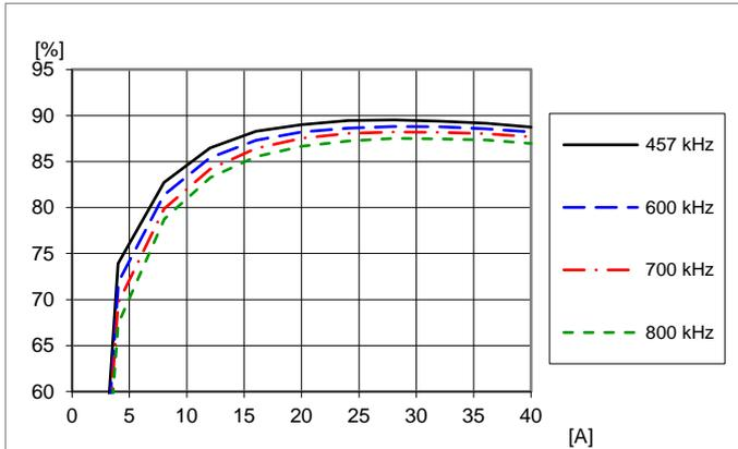
Efficiency vs. load current and switching frequency at  $V_I = 12\text{ V}$ ,  $V_O = 1.0\text{ V}$ ,  $C_O = 4 \times 330\text{ }\mu\text{F}/10\text{ m}\Omega + 10 \times 100\text{ }\mu\text{F}$ . Frequency changed by PMBus command FREQUENCY\_SWITCH.
