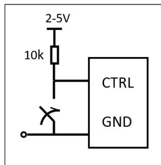
The product is equipped with remote control function. The CTRL pin polarity can be configured active high or active low using PMBus command ON\_OFF\_CONFIG. In active high (positive) mode, CTRL pin requires a pullup resistor to a DC supply to turn on the module. Turn off is achieved by connecting the CTRL pin to GND. And active low (negative) vice versa.
