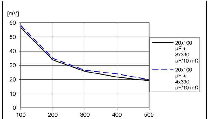
Load transient peak voltage deviation vs. ASCR gain and external capacitance. Step (20–60–20 A).  $V_I = 12\text{ V}$ ,  $V_O = 1.0\text{ V}$ ,  $f_{sw} = 457\text{ kHz}$ , ASCR residual = 82,  $di/dt = 2\text{ A}/\mu\text{s}$ . ASCR gain changed by PMBus command ASCR\_CONFIG.
