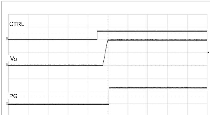
Output enabled by CTRL pin.  $V_i = 12\text{ V}$ ,  $I_o = 40\text{ A}$ .
