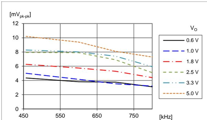
Output voltage ripple  $V_{pk-pk}$  vs. switching frequency at  $V_I = 12\text{ V}$ ,  $I_O = \text{max } I_O$ ,  $C_O = 4 \times 330\text{ }\mu\text{F}/10\text{ m}\Omega + 10 \times 100\text{ }\mu\text{F}$ . Frequency changed by PMBus command FREQUENCY\_SWITCH.
