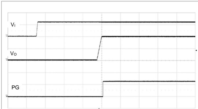
Output enabled by applying  $V_i$ .  $V_i = 12\text{ V}$ ,  $I_o = 40\text{ A}$ .
