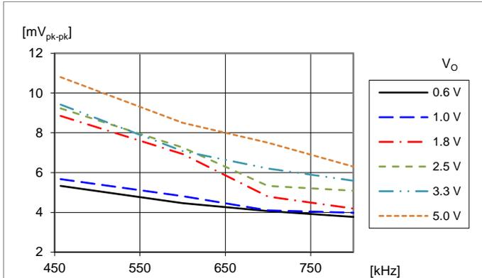
Output voltage ripple  $V_{pk-pk}$  vs. switching frequency at  $V_I = 12\text{ V}$ ,  $I_O = \text{max } I_O$ ,  $C_O = 8 \times 330\text{ }\mu\text{F}/10\text{ m}\Omega + 20 \times 100\text{ }\mu\text{F}$ . Frequency changed by PMBus command FREQUENCY\_SWITCH.
