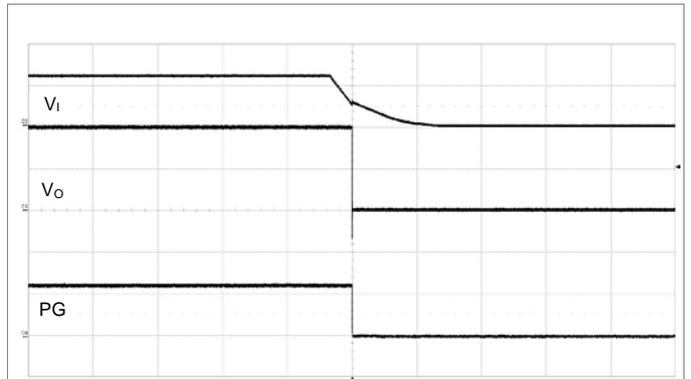
Output disabled by removing  $V_i$ .  $V_i = 12\text{ V}$ ,  $I_o = 80\text{ A}$ .
