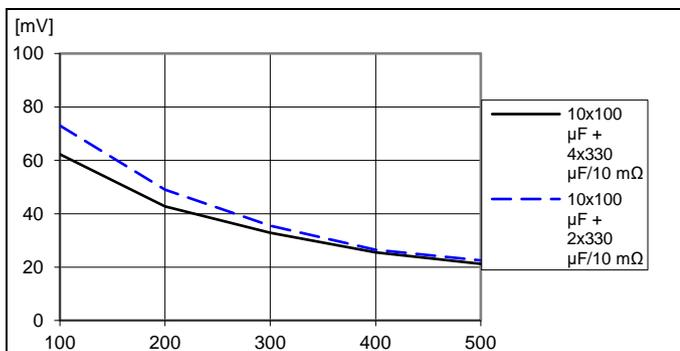
Load step 10-30-10 A, di/dt = 2 A/μs.
