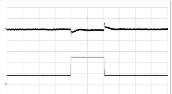
Output voltage response to load current step change (25%–75%–25%) at  $V_I = 12\text{ V}$ ,  $C_{OUT} = 8 \times 330\text{ }\mu\text{F}/10\text{ m}\Omega + 20 \times 100\text{ }\mu\text{F}$ ,  $di/dt = 2\text{ A}/\mu\text{s}$ ,  $ACSR\text{ Gain} = 219$  and  $ASCR\text{ Residual} = 82$ .
