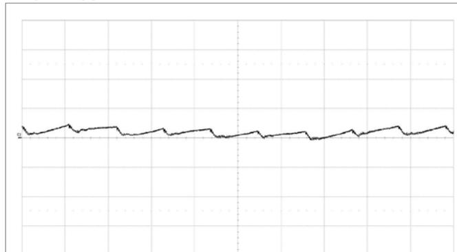
Fundamental output voltage ripple at  $V_I = 12\text{ V}$ ,  $I_O = 40\text{ A}$ ,
