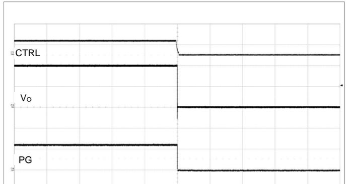
Output disabled by CTRL pin.  $V_i = 12\text{ V}$ ,  $I_o = 80\text{ A}$ .
