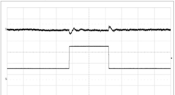
Output voltage response to load current step change (25%–75%–25%) at  $V_I = 12\text{ V}$ ,  $C_{OUT} = 8 \times 330\text{ }\mu\text{F}/10\text{ m}\Omega + 20 \times 100\text{ }\mu\text{F}$ ,  $di/dt = 2\text{ A}/\mu\text{s}$ ,
