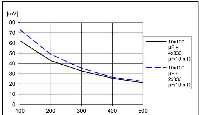
Load transient peak voltage deviation vs. ASCR gain and external capacitance. Step (10–30–10 A).  $V_I = 12\text{ V}$ ,  $V_O = 1.0\text{ V}$ ,  $f_{sw} = 457\text{ kHz}$ ,  $\text{ASCR residual} = 82$ ,  $di/dt = 2\text{ A}/\mu\text{s}$ . ASCR gain changed by PMBus command ASCR\_CONFIG.
