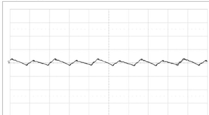
Fundamental output voltage ripple at  $V_I = 12\text{ V}$ ,  $I_O = 70\text{ A}$ ,  $C_{OUT} = 8 \times 330\text{ }\mu\text{F}/10\text{ m}\Omega + 20 \times 100\text{ }\mu\text{F}$
