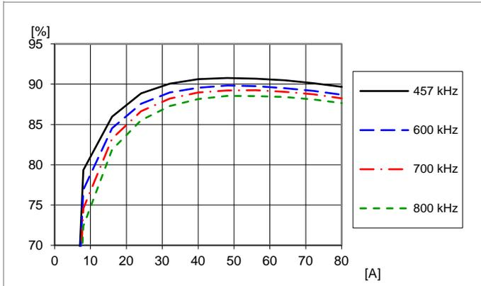
Efficiency vs. load current and switching frequency at  $V_I = 12\text{ V}$ ,  $V_O = 1.0\text{ V}$ ,  $C_O = 8 \times 330\text{ }\mu\text{F}/10\text{ m}\Omega + 20 \times 100\text{ }\mu\text{F}$ . Frequency changed by PMBus command FREQUENCY\_SWITCH.
