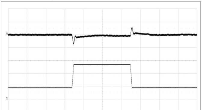
Output voltage response to load current step change (25%–75%–25%) at  $V_I = 12\text{ V}$ ,  $C_{OUT} = 8 \times 330\text{ }\mu\text{F}/10\text{ m}\Omega + 20 \times 100\text{ }\mu\text{F}$ ,  $di/dt = 2\text{ A}/\mu\text{s}$ ,  $ACSR\ Gian=219$  and  $ASCR\ Residual=82$ .
