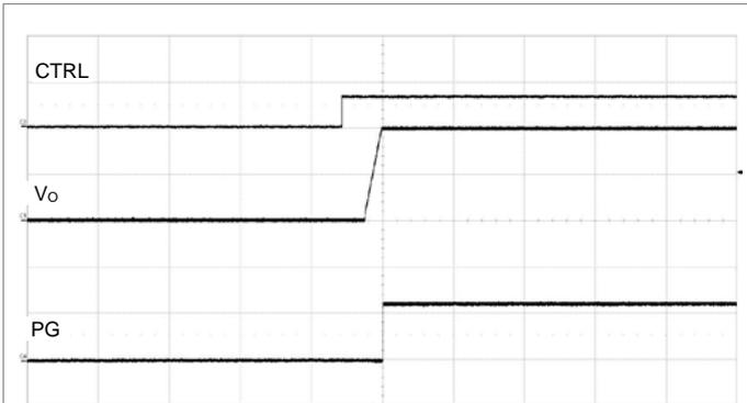
Output enabled by CTRL pin.  $V_i = 12\text{ V}$ ,  $I_o = 80\text{ A}$ .
