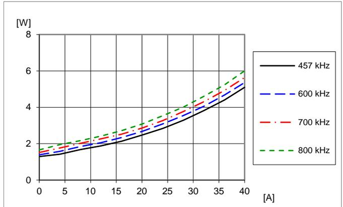
Dissipated power vs. load current and switching frequency at  $V_I = 12\text{ V}$ ,  $V_O = 1.0\text{ V}$ ,  $C_O = 4 \times 330\text{ }\mu\text{F}/10\text{ m}\Omega + 10 \times 100\text{ }\mu\text{F}$ . Frequency changed by PMBus command FREQUENCY\_SWITCH.
