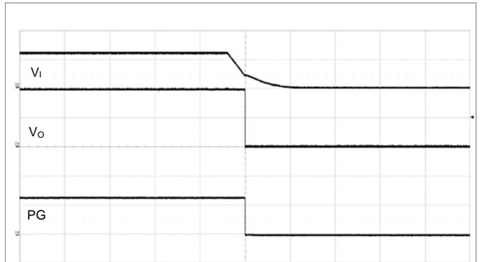
Output disabled by removing  $V_i$ .  $V_i = 12\text{ V}$ ,  $I_o = 40\text{ A}$ .
