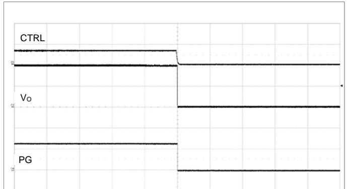
Output disabled by CTRL pin.  $V_i = 12\text{ V}$ ,  $I_o = 40\text{ A}$ .
