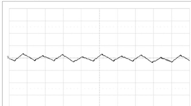
Fundamental output voltage ripple at  $V_I = 12\text{ V}$ ,  $I_O = 65\text{ A}$ ,  $C_{OUT} = 8 \times 330\text{ }\mu\text{F}/10\text{ m}\Omega + 20 \times 100\text{ }\mu\text{F}$
