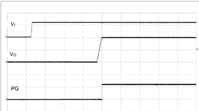
Output enabled by applying  $V_i$ .  $V_i = 12\text{ V}$ ,  $I_o = 80\text{ A}$ .
