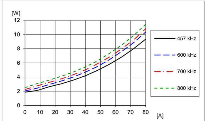
Dissipated power vs. load current and switching frequency at  $V_I = 12\text{ V}$ ,  $V_O = 1.0\text{ V}$ ,  $C_O = 8 \times 330\text{ }\mu\text{F}/10\text{ m}\Omega + 20 \times 100\text{ }\mu\text{F}$ . Frequency changed by PMBus command FREQUENCY\_SWITCH.
