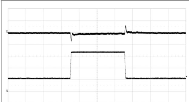
Output voltage response to load current step change (25%–75%–25%) at V_i = 12\text{ V} , C_{OUT} = 4 \times 330\text{ }\mu\text{F}/10\text{ m}\Omega + 12 \times 100\text{ }\mu\text{F} , di/dt = 2\text{ A}/\mu\text{s} , ACSR Gain=200 and ASRC Residual=90. Scale from top: 50 mV/div, 10 A/div, 200 \mu\text{s} /div. Note: Sense pins are connected to load.
