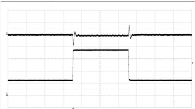
Output voltage response to load current step change (25%–75%–25%) at V_i = 12 V , C_{OUT} = 2 \times 330 \mu F / 10 m\Omega + 6 \times 100 \mu F , di/dt = 2 A/\mu s , ACSR Gian=200 and ASCR Residual=90. Scale from top: 50 mV/div, 5 A/div, 200 \mu s /div. Note: Sense pins are connected to load.
