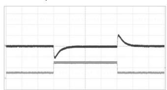
Output voltage response to output current change (10-30-10 A) at  $V_1$ =12V,  $C_0$ =5 x 100  $\mu$ F ceramic + 4 x 470  $\mu$ F POSCAP (ESR 10 m $\Omega$ ),  $T_{P1}$  = +25°C, di/dt=2A/ $\mu$ s.
