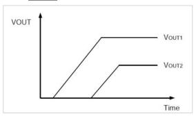
Figure 8: Illustration of output voltage sequencing
