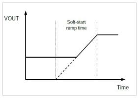
Figure 7: Illustration of pre-bias startup
