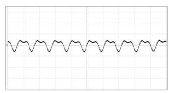
Output voltage ripple at  $V_i$ =12V,  $I_o$ =max  $I_o$ ,  $T_{P1}$  = +25 $^{\circ}$ C Scale: 10 mV/div, 2  $\mu$ s/div, 20 MHz bandwidth
