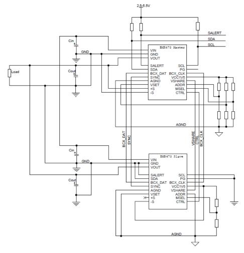
Figure 10: circuit diagram for 2 parallel operation
