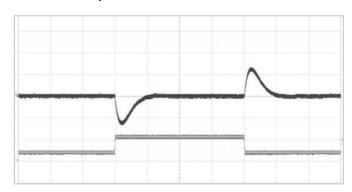
Output voltage response to output current change (7.5-22.5-7.5 A) at V<sub>i</sub>=12V, C<sub>O</sub>=5 x 100  $\mu$ F ceramic + 4 x 470  $\mu$ F POSCAP (ESR 10 m $\Omega$ ),  $T_{P1}$  = +25°C, di/dt=2A/ $\mu$ s.
