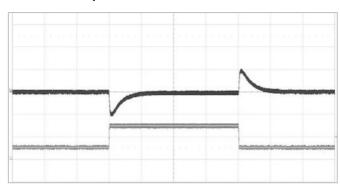
Output voltage response to output current change (10-30-10 A) at  $V_1$ =12V,  $C_0$ =8 x 100  $\mu$ F ceramic + 4 x 470  $\mu$ F POSCAP (ESR 10 m $\Omega$ ),  $T_{P1}$  = +25°C, di/dt=2A/ $\mu$ s.
