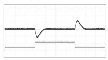
Output voltage response to output current change (7.5-22.5-7.5 A) at V<sub>I</sub>=12V, C<sub>O</sub>=8 x 100  $\mu$ F ceramic + 4 x 470  $\mu$ F POSCAP (ESR 10 m $\Omega$ ), T<sub>P1</sub> = +25°C, di/dt=2A/ $\mu$ s.
