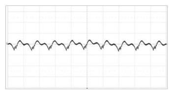
Output voltage ripple at  $V_i$ =12V,  $I_o$ =max  $I_o$ ,  $T_{P1}$  = +25°C Scale: 5 mV/div, 2  $\mu$ s/div, 20 MHz bandwidth
