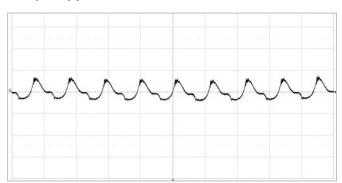
Output voltage ripple at  $V_i$ =12V,  $I_o$ =max  $I_o$ ,  $T_{P1}$  = +25°C Scale: 5 mV/div, 2  $\mu$ s/div, 20 MHz bandwidth
