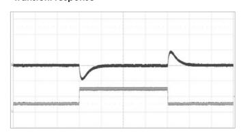
Output voltage response to output current change (10-30-10 A) at  $V_i$ =12V,  $C_o$ =8 x 100  $\mu$ F ceramic + 4 x 470  $\mu$ F POSCAP (ESR 10 m $\Omega$ ),  $T_{P1}$  = +25°C, di/dt=2A/ $\mu$ s.
