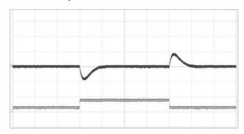
Output voltage response to output current change (5-15-5 A) at  $V_1$ =12V,  $C_0$ =5 x 100  $\mu$ F ceramic + 4 x 470  $\mu$ F POSCAP (ESR 10 m $\Omega$ ),  $T_{P1}$  = +25°C, di/dt=2 $A/\mu$ s.
