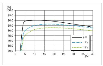
Efficiency vs. output current at T<sub>P1</sub> = +25°C
