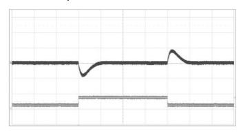
Output voltage response to output current change (5-15-5 A) at  $V_1$ =12V,  $C_0$ =8 x 100  $\mu$ F ceramic + 4 x 470  $\mu$ F POSCAP (ESR 10 m $\Omega$ ),  $T_{P1}$  = +25°C, di/dt=2A/ $\mu$ s.
