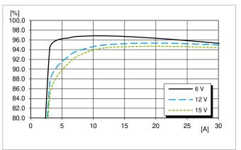
Efficiency vs. output power and input voltage at T<sub>P1</sub> = +25°C
