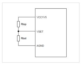
Figure 3: Pin-strap resistor for VSET pin
