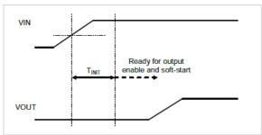
Figure 13: Illustration of Initialization time
