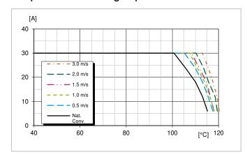
Available output current vs. ambient air temperature and airflow, V<sub>i</sub>=12V, V<sub>O</sub>=1.8V.
