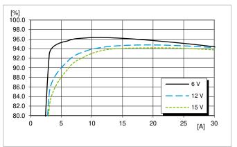
Efficiency vs. output power and input voltage at T<sub>P1</sub> = +25°C
