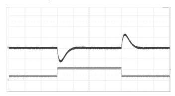
Output voltage response to output current change (7.5-22.5-7.5 A) at V<sub>I</sub>=12V, C<sub>O</sub>=5 x 100  $\mu$ F ceramic + 4 x 470  $\mu$ F POSCAP (ESR 10 m $\Omega$ ), T<sub>P1</sub> = +25°C, di/dt=2A/ $\mu$ s.
