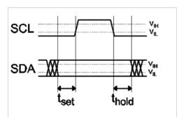
Picture 12: Set-up and hold times timing diagramm
