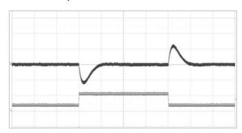
Output voltage response to output current change (7.5-22.5-7.5 A) at V<sub>i</sub>=12V, C<sub>O</sub>=8 x 100  $\mu$ F ceramic + 4 x 470  $\mu$ F POSCAP (ESR 10 m $\Omega$ ),  $T_{P1}$  = +25°C, di/dt=2A/ $\mu$ s.
