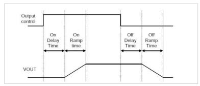
Figure 6: Illustration of soft-start and soft-stsop
