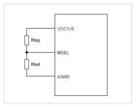
Figure 5: Pin-strap resistor for MSEL pin
