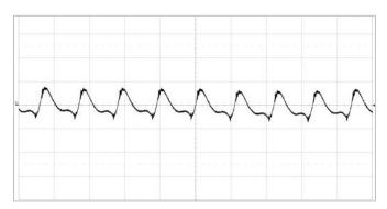
Output voltage ripple at  $V_1=12V$ ,  $I_0=\max I_0$ ,  $T_{P1}=+25^{\circ}C$  Scale: 5 mV/div, 2  $\mu$ s/div, 20 MHz bandwidth
