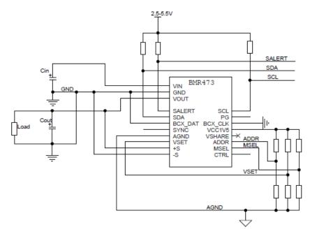
Figure 9: Circuit diagram for standalone operation
