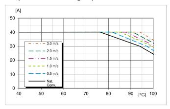
Available output current vs. ambient air temperature and airflow, V;=12V, Vo=0.6V.
