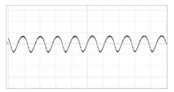
Output voltage ripple at  $V_1$ =12V,  $I_0$ =max  $I_0$ ,  $T_{P1}$  = +25 $^{\circ}$ C Scale: 10 mV/div, 2  $\mu$ s/div, 20 MHz bandwidth
