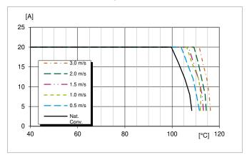
Available output current vs. ambient air temperature and airflow, V = 12V, V = 3.3V.
