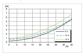
Dissipated power vs. load current at T<sub>P1</sub> = +25°C
