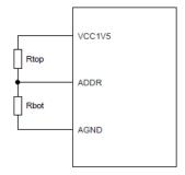
Figure 11: PMBus addressing with pin strap
