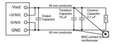
Figure 4: Output ripple and noise test set-up
