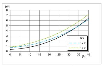
Dissipated power vs. load power at  $T_{P1} = +25$ °C
