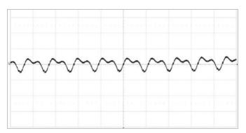
Output voltage ripple at  $V_I=12V$ ,  $I_0=\max I_0$ ,  $T_{P1}=+25^{\circ}C$  Scale: 10 mV/div, 2  $\mu$ s/div, 20 MHz bandwidth
